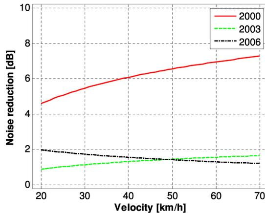
Fig. 2. The decrease in the acoustic effectiveness of the porous pavement (Pavement A).
