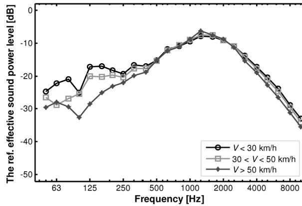
Fig. 3. The referenced level of the effective sound power on conventional asphalt (2000, Pavement A).
