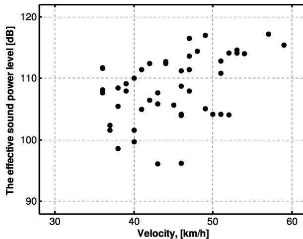
Fig. 6. The effective sound power level  $\tilde{L}_{WA}$  of heavy vehicles versus vehicle speed  $V$  on conventional asphalt.
