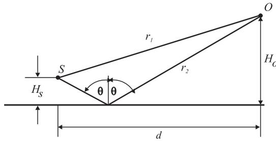
Fig. 8. The source – receiver geometry in the horizontal plane.
