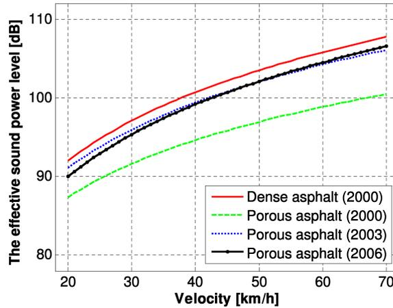
Fig. 1. The effective sound power level  $\tilde{L}_{WA}$  versus vehicle speed  $V$  on conventional asphalt, new porous asphalt and porous asphalt after three and six years of use (Pavement A).
