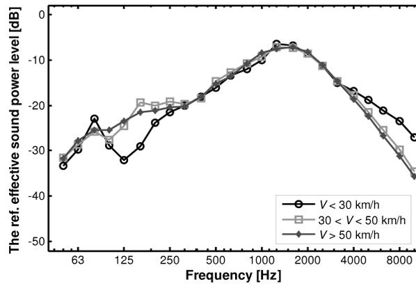
Fig. 5. The referenced level of the effective sound power on porous pavement after three years of use (2003, Pavement A).
