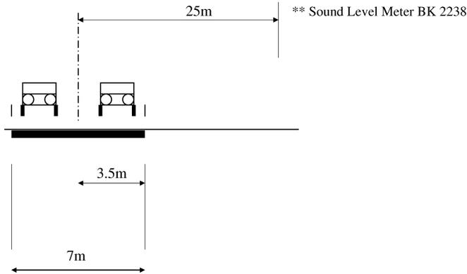
Fig. 1. Illustration of the road (BR 416) and the positioning of the sound level meter.
