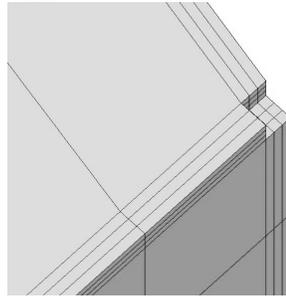
Fig. 2. FEM mesh near corner of the cage.
