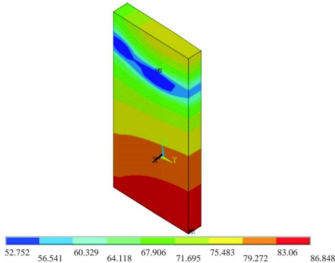
Fig. 5. The sound pressure level in the vertical cross-section ( $x = 0.7$  m) for the second resonance frequency (activated piezoelectric elements).
