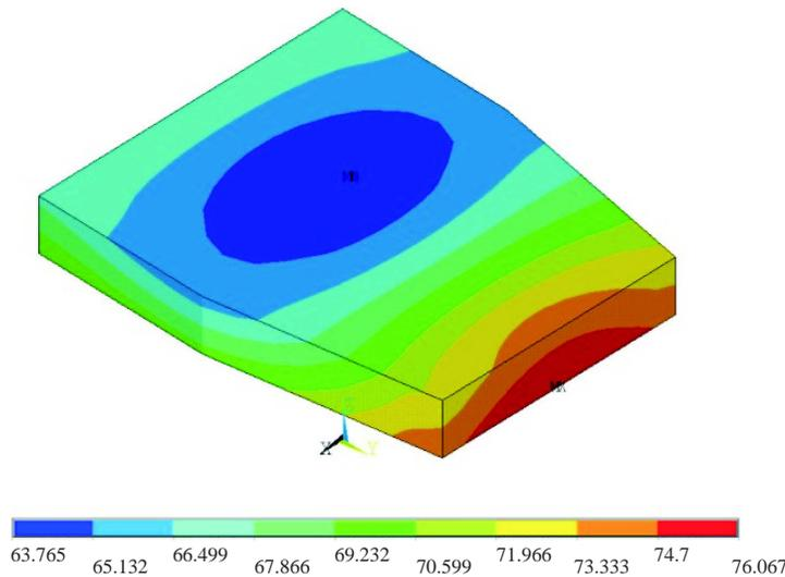
Fig. 6. The sound pressure level in the horizontal cross-section ( $z = 0.7$  m) for the second resonance frequency (activated piezoelectric elements).
