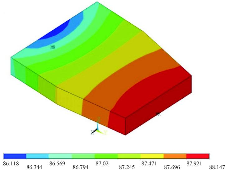
Fig. 4. The sound pressure level in the horizontal cross-section ( $z = 0.7$  m) for the first resonance frequency (non activated piezoelectric elements).
