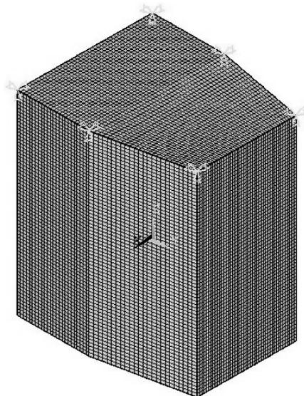
Fig. 1. FEM model of the crane cage.
