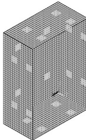
Fig. 3. Distribution of piezoelectric elements.
