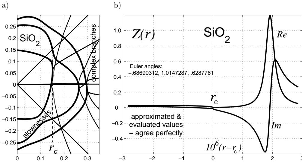
Fig. 1. a) Eigenvalues dependent on the wave-number  $r$  (horizontal axis) draw the slowness curves when they are real-valued; they are complex-valued above cut-off wave-numbers of bulk waves (the lowest one,  $r_c$ , is marked in the figure); b) Resonant behavior of the surface impedance  $Z(r)$  in small domain around  $r_c$ ; the approximated values evaluated using the method of [4] remain in perfect agreement within this important domain of wave-number  $r$ .
