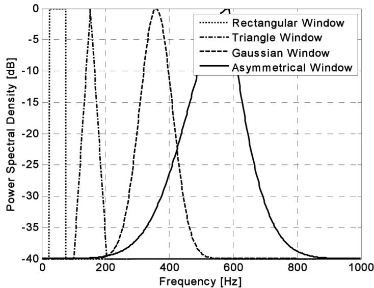
Fig. 3. Window-type magnitude of the generalised disturbance PSD.
