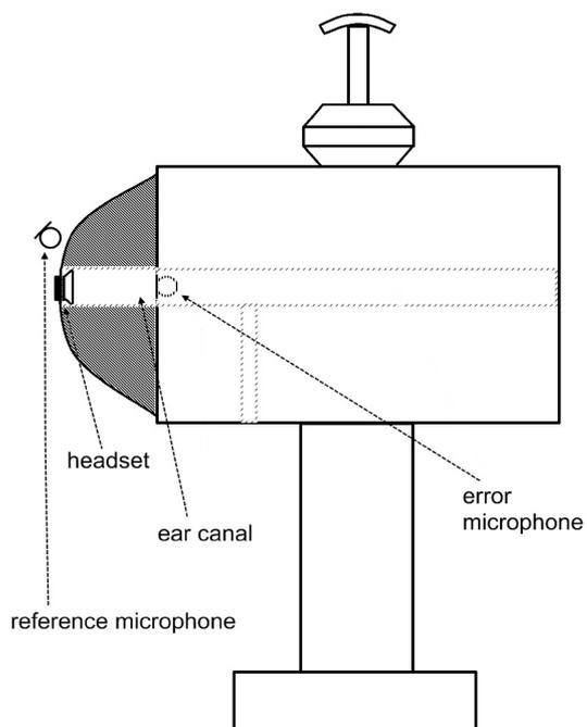
Fig. 4. Artificial head with active headset.
