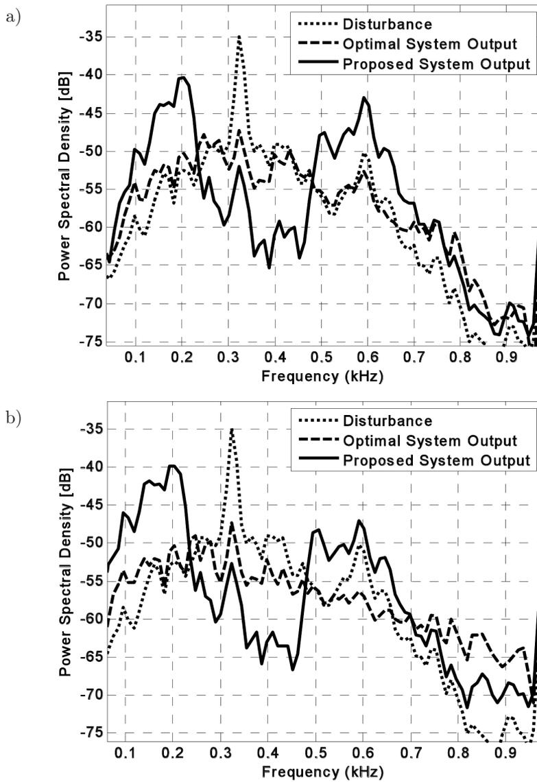
Fig. 9. Control results for the optimal and proposed systems (triangular window disturbance PSD) a) IMC structure; b) feedforward structure.
