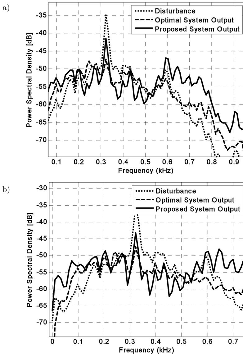
Fig. 10. Control results for the optimal and proposed systems (asymmetrical Gaussian window disturbance PSD) a) IMC structure; b) feedforward structure.
