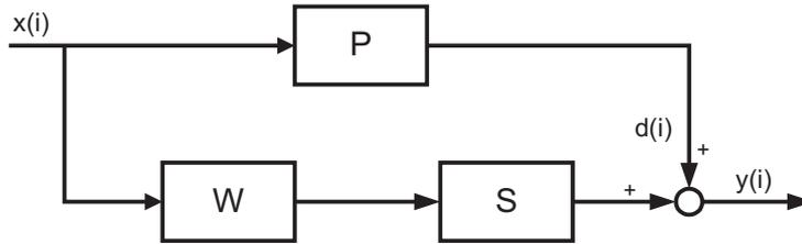
Fig. 1. Feedforward structure.
