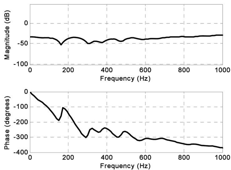
Fig. 5. Frequency response of the plant model.
