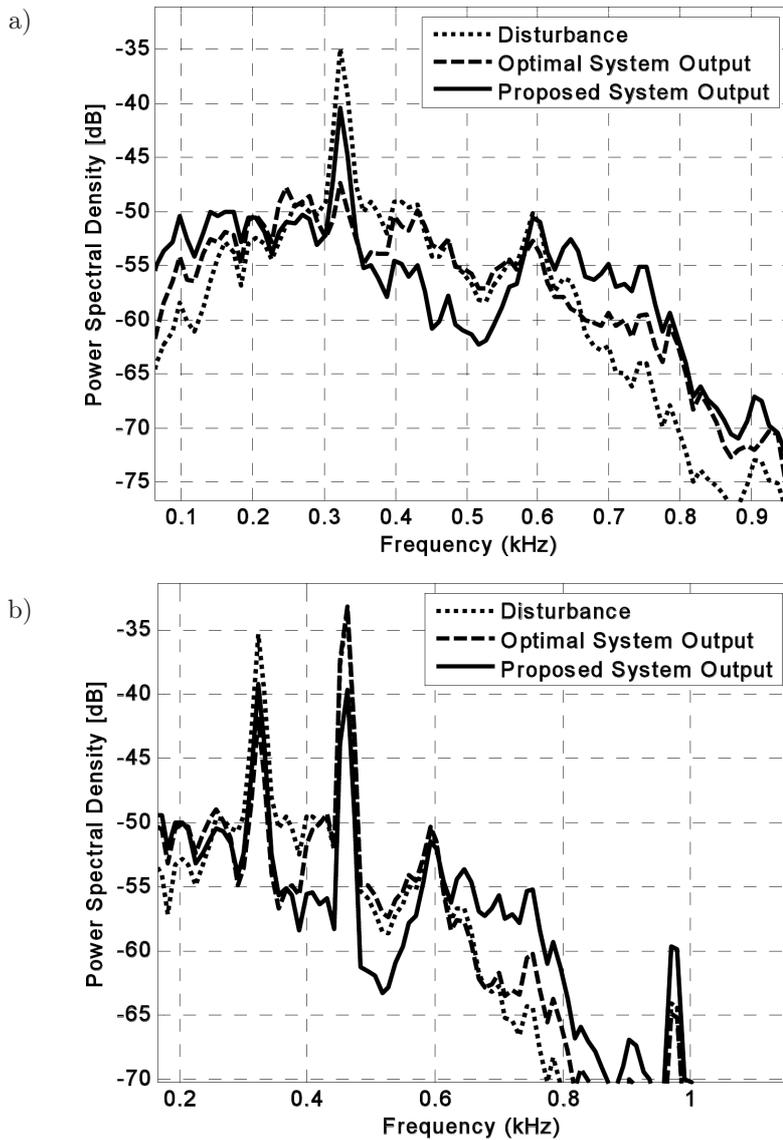
Fig. 8. Control results for the optimal and proposed systems in the IMC structure (Gaussian window disturbance PSD) operating: a) for the disturbance used in design process; b) for the disturbance with additional components at 440–470 Hz.
