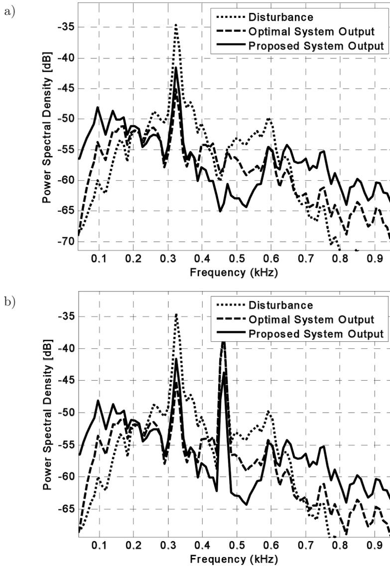
Fig. 7. Control results for the optimal and proposed systems in the feedforward structure (Gaussian window disturbance PSD) operating: a) for the disturbance used in design process; b) for the disturbance with additional components at 440–470 Hz.
