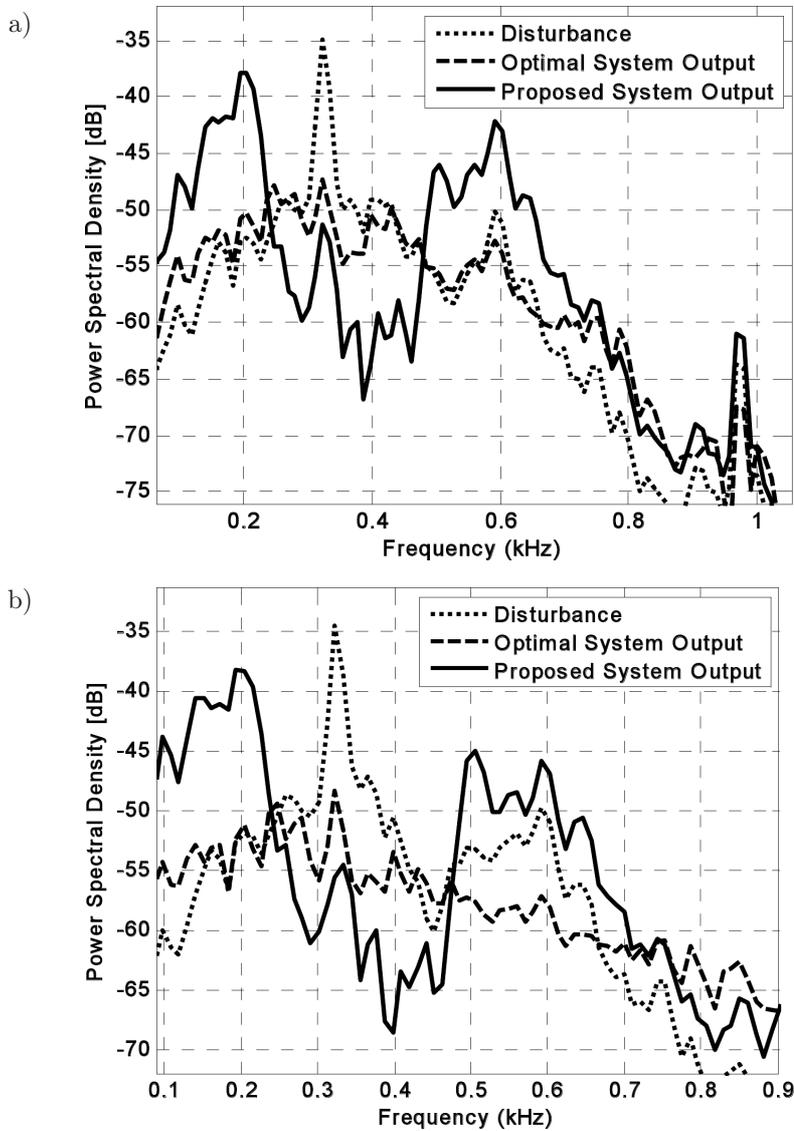
Fig. 6. Control results for the optimal and proposed systems (rectangular window disturbance PSD) a) IMC structure; b) feedforward structure.
