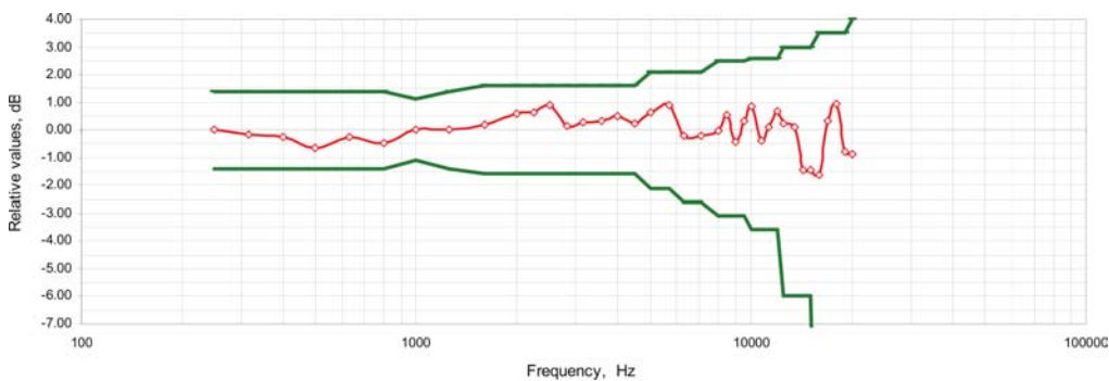
Fig. 2. An example of frequency responses of the omni-directional microphone for the reference direction 0^\circ . Green lines mark the limit of permissible errors, acc. to [2].
