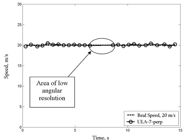
Fig. 12. Source speed obtained by processing results of ULA-7 with antenna perpendicular to the vehicle travelling line for assumption 2.
