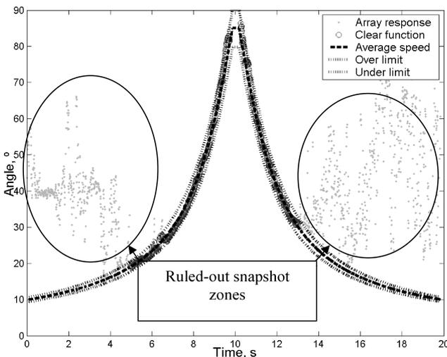
Fig. 7. The zones bounded by the vehicles average speed rule out points giving no information on sound source localization, ‘clean function’.
