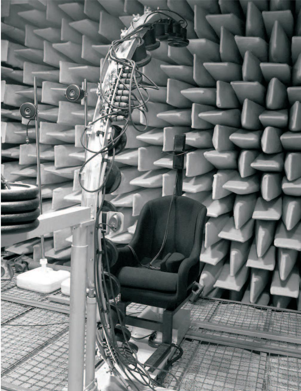
Fig. 1. Overview of the HRTF measurement equipment.
