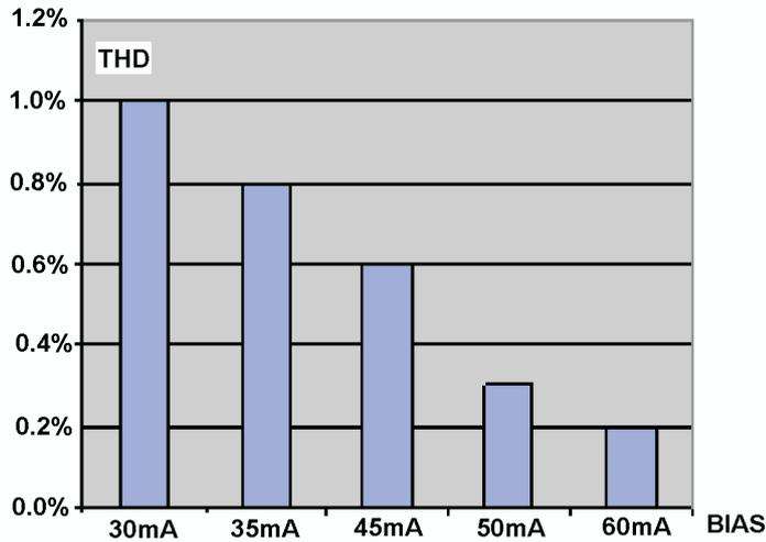
Fig. 3. Nonlinear distortion in function of current for EL34 tubes, with  $P = 30 \text{ W}$ .
