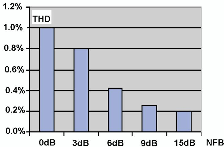
Fig. 4. Nonlinear distortions in function of depth of NFB for EL34 tube, with  $P = 30$  W.
