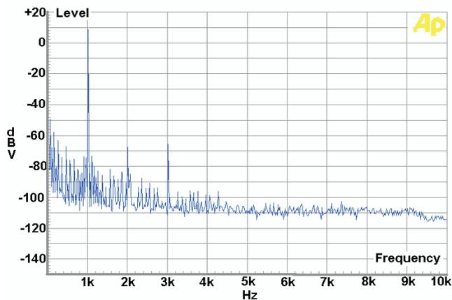
Fig. 7. Harmonics content in the signal for  $P = 1$  W at 1 kHz.
