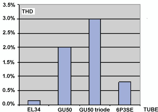
Fig. 2. Nonlinear distortions as depending on the types of power stage tubes and work circuit for  $P = 10$  W.
