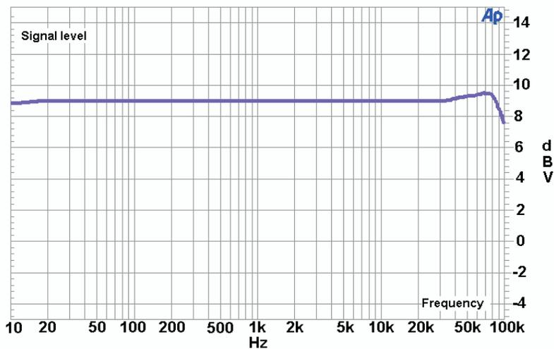
Fig. 5. Pass band –15 dB negative feedback for EL34 tube, with  $P = 1$  W.
