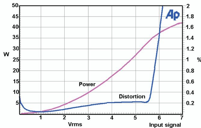
Fig. 6. Power and distortions characteristics in the function of input voltage.
