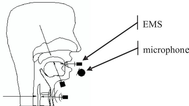
Fig. 3. Sensors' configuration in relation to a patient's head.
