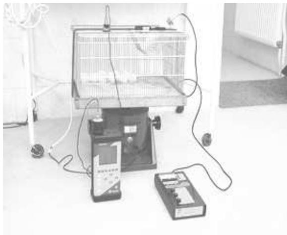
Fig. 1. Experimental set-up. Vibration-generating circuit and control and analysis circuit.
