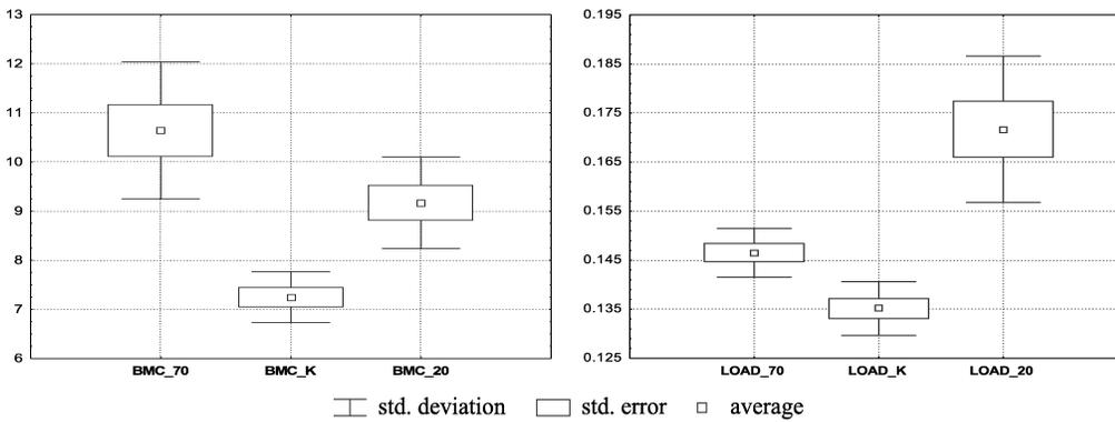
Fig. 13. The effects of vibrations to BMC [g]. Fig. 14. The effects of vibrations on load at yield –  $F$  [kN].
