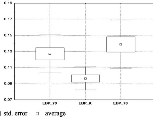
Fig. 15. The effects of vibrations on displacement at yield –  $s$  [mm].
