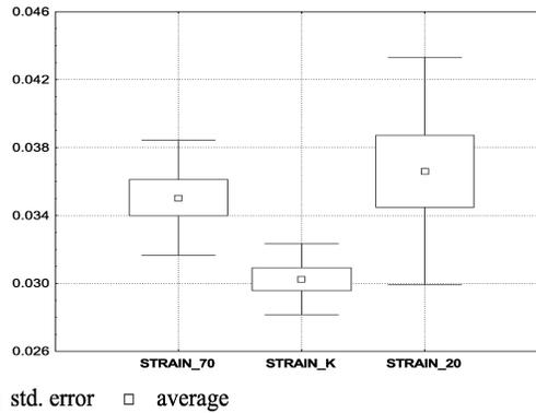
Fig. 18. The effects of vibrations on strain at yield –  $\varepsilon$  [-].
