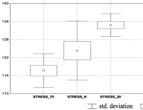
Fig. 17. The effects of vibrations on Stress at yield –  $\sigma_g$  [MPa].
