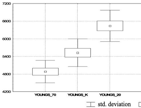
Fig. 19. The effects of vibrations on Young's modulus –  $E$  [MPa].
