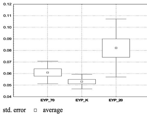
Fig. 20. The effects of vibrations on energy to yield point –  $EYP$  [J].
