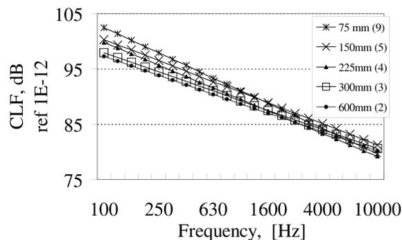
Fig. 8. Experimental CLFs for point screw-bolts junctions, variety of density of joining screw.
