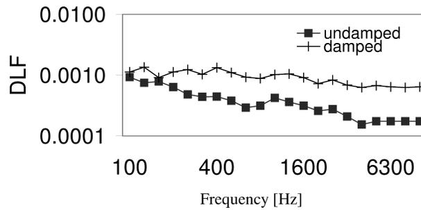
Fig. 4. DLFs of steel plate damper on circumferences and undamped, thickness 0.001 [m].
