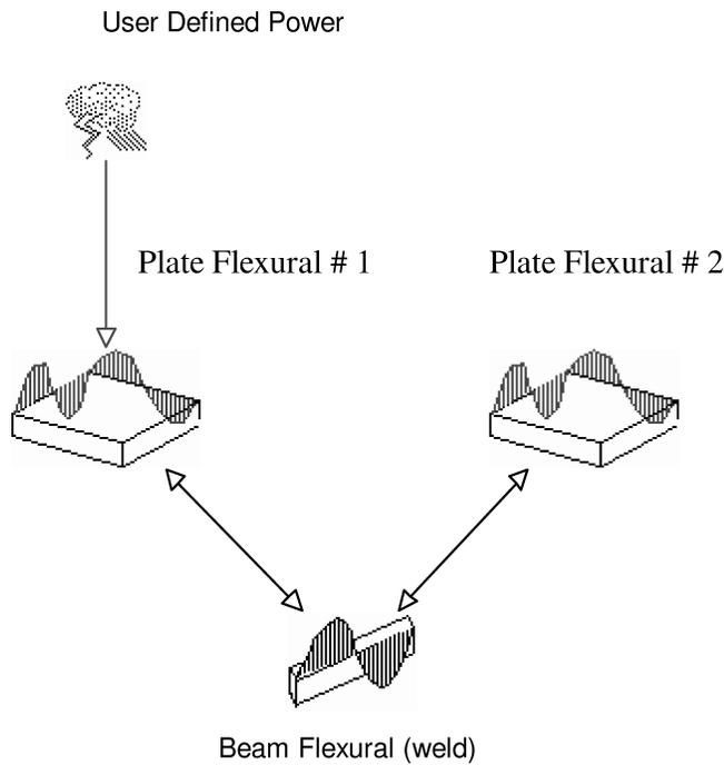
Fig. 2a. SEA model: line-welded junction.
