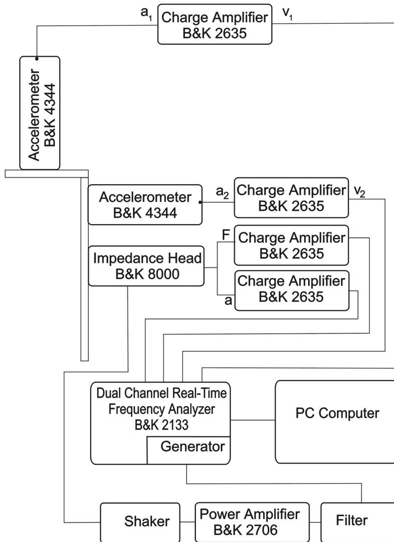
Fig. 3. Measurement set-up.
