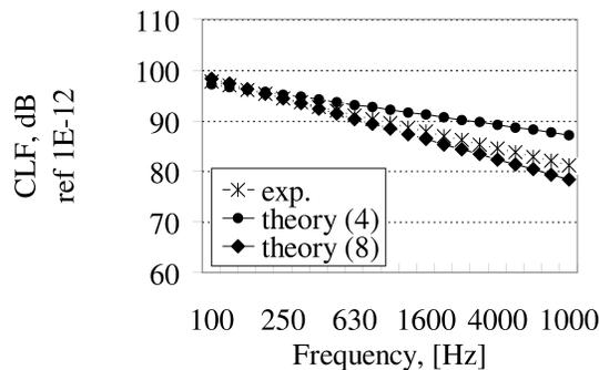
Fig. 6. Experimental and theory CLFs (Eq. (4) and Eq. (8)) for weld joined plates, thickness ratio 1.5:1.
