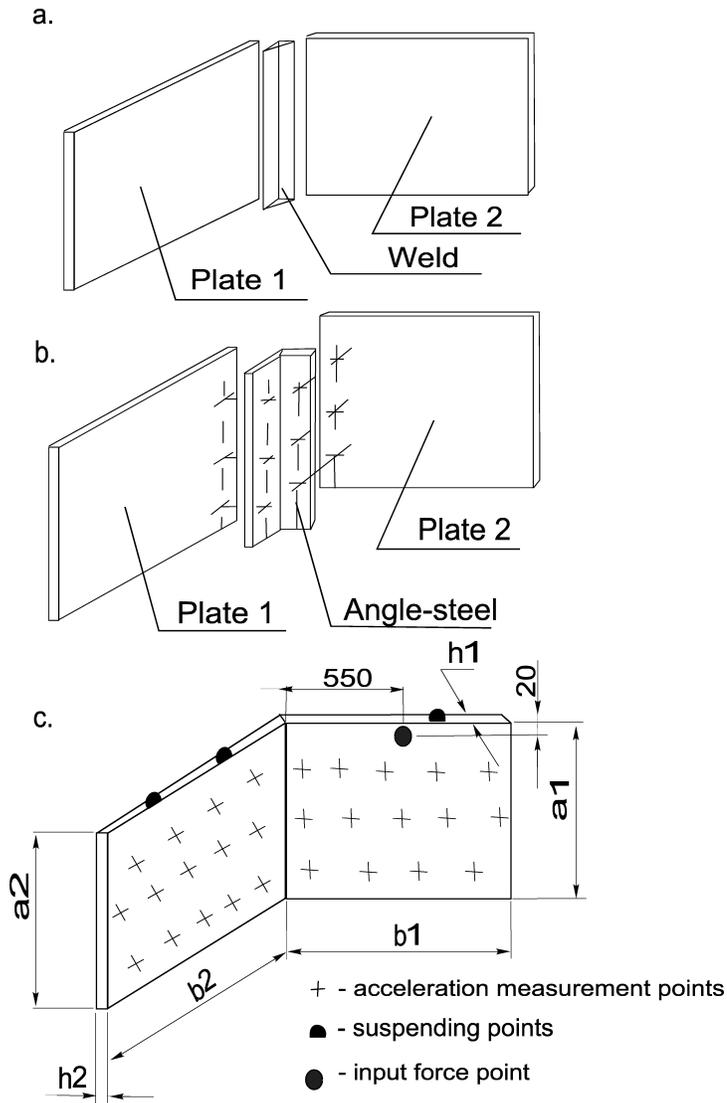
Fig. 1. Plate connections: a) line-welded, b) point with angle steel, c) distribution of measurement, suspended and input force points in plates.
