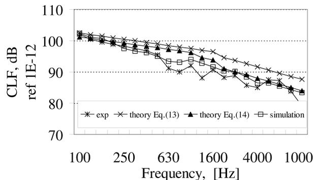
Fig. 9. An example of experimental, theory Eq. (13), (14) and simulated CLFs for spot welded junction, nine joining points, distance of spot welds  $l = 0.075$ [m].
