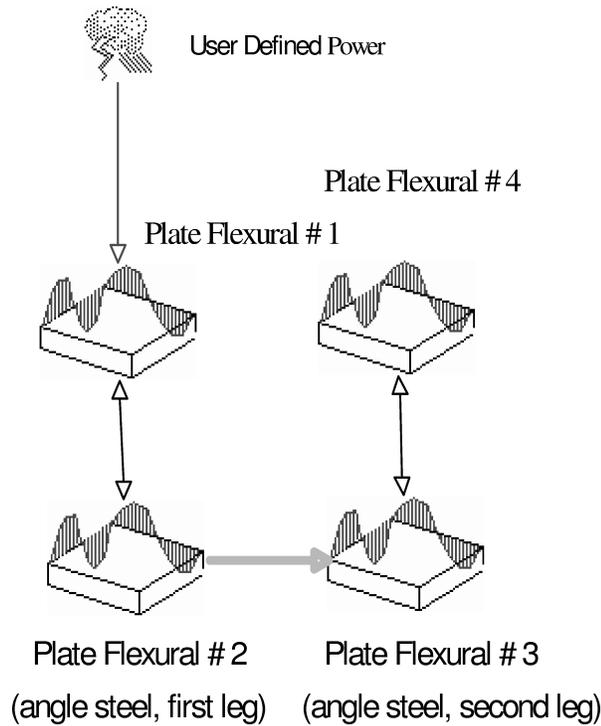
Fig. 2b. SEA model: point type junction.
