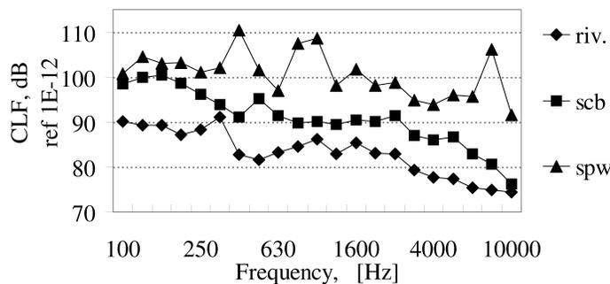
Fig. 10. Experimental CLFs for point junctions: screw-bolts, rivets and spot welded.
