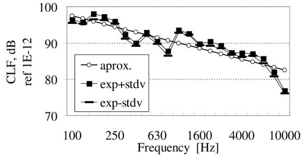
Fig. 5. Experimental values of CLFs for plates joined with weld thickness 0.0004[m], thickness ratio 3:1 (0.003[m] and 0.001[m]).
