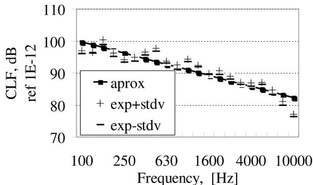
Fig. 7. Experimental CLFs for point screw-bolts junctions' plates: five joining screws, distance of screws 0.300[m].
