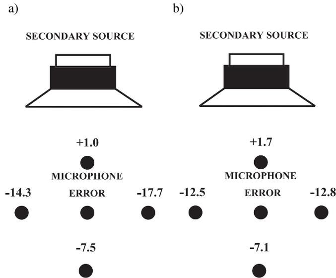
Fig. 8. Silence area created by the ANR systems: a) white noise filtered by the third filter  $f_0 = 125$  Hz, b) white noise filtered by the octave filter  $f_0 = 125$  Hz.
