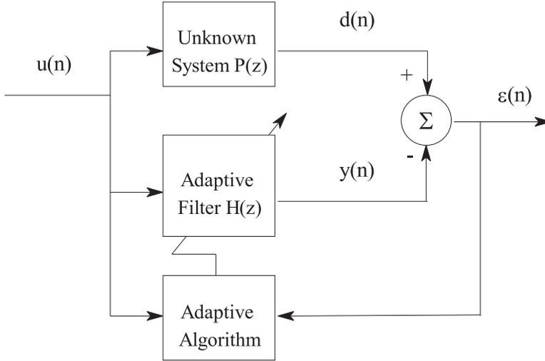
Fig. 1. Block diagram of the adaptive control system.
