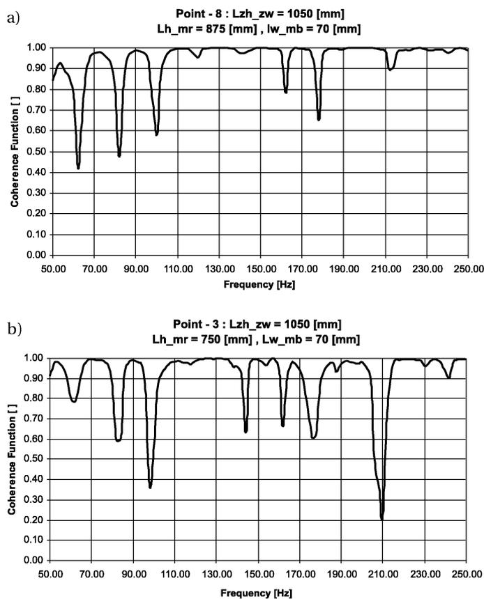
Fig. 7. Coherence function between the reference and error microphones for different locations of sensors in the room.
