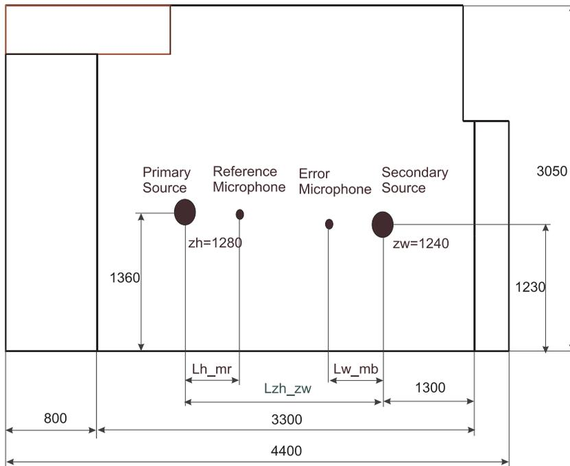
Fig. 6. Location of microphones and sources in the room.
