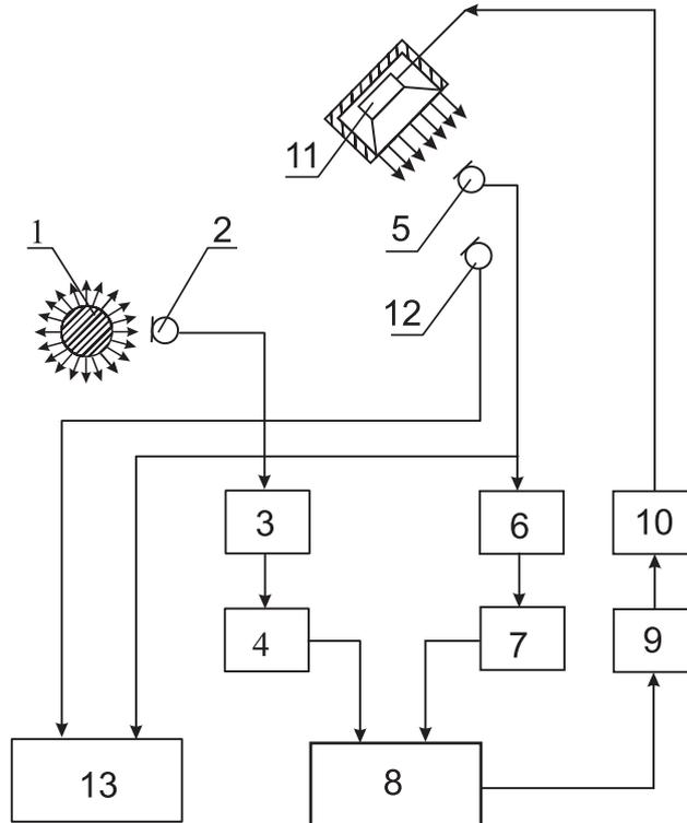
Fig. 2. Block diagram of the active noise reduction system.
