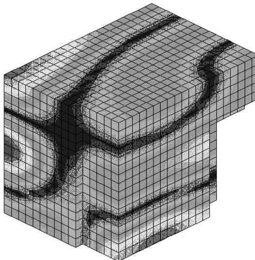
Fig. 5. Graphical representation of the sound pressure distribution at mode frequency 123.552 Hz.
