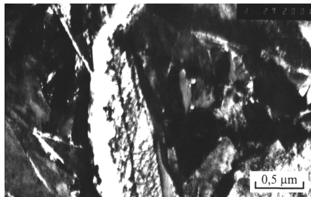
Fig. 6. A microstructure of bainite sheaves of butterfly morphology with the etched midrib after austempering at 160°C, 3000 s.
