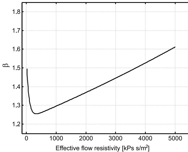
Fig. 3. Changes in the  $\beta$  parameter as a function of the effective flow resistivity  $\sigma$ .
