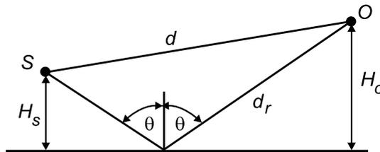
Fig. 1. Source – receiver geometry in the horizontal plane.
