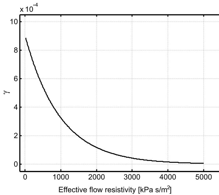
Fig. 4. Changes in the  $\gamma$  parameter as a function of the effective flow resistivity  $\sigma$ .
