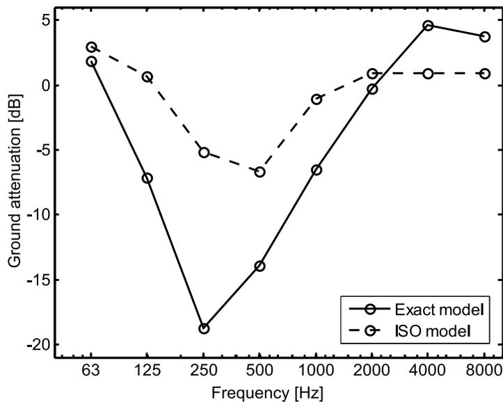
Fig. 6. The ground attenuation calculated using the exact model of the ground effect and ISO 9613 ( $d = 40$  m,  $H_s = 0.5$  m,  $H_o = 1.2$  m,  $\sigma = 25$  kPa s/m<sup>2</sup>).
