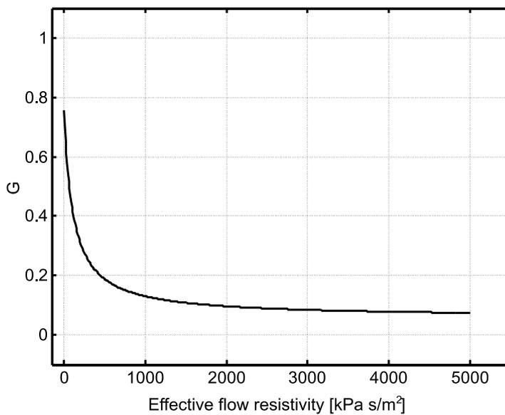
Fig. 7. Changes in the ground factor  $G$  as a function of the effective flow resistivity  $\sigma$  (Eq. (30), Table 3).
