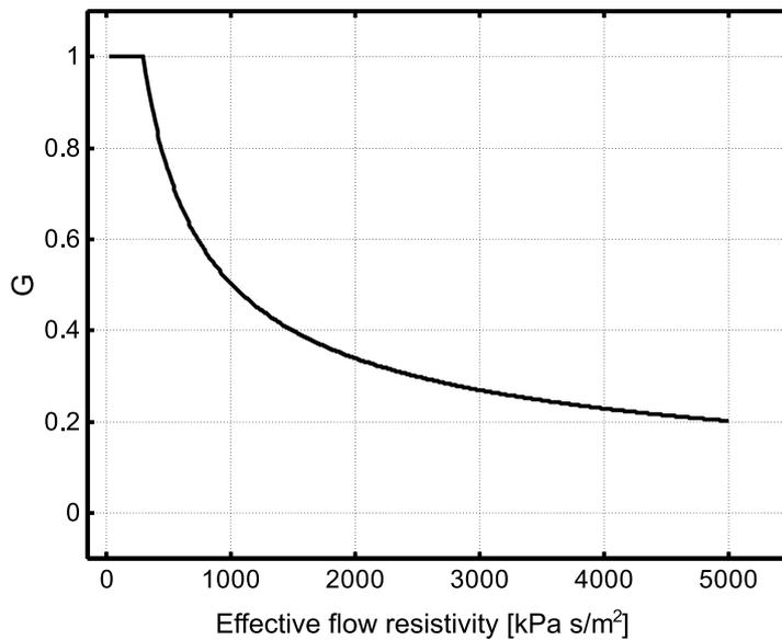
Fig. 5. Changes in the ground factor  $G$  calculated using Eq. (29).
