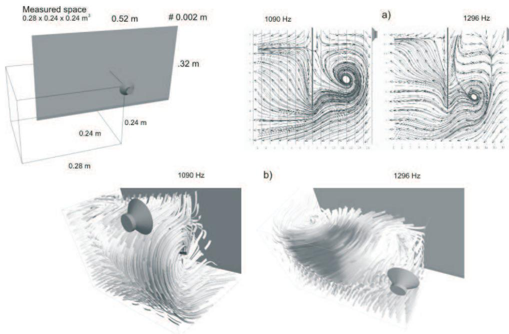
Fig. 3. Experimental set-up and distribution of intensity streamlines in the plane of symmetry axis of measured space (a), and intensity streamlines around a one corner of thin (2 mm) plate.
