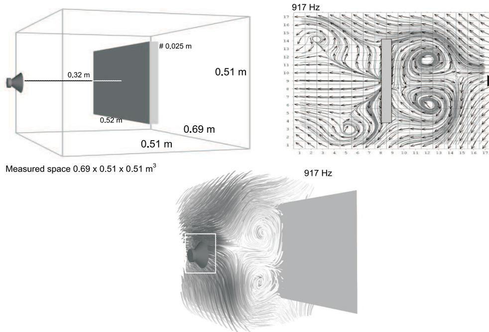
Fig. 1. The geometry of experimental set-up and distribution of intensity streamlines in the plane of symmetry axis of the plate (2D) and in 1/2 space of measurement (3D). Source is 0.6 m from obstacle.
