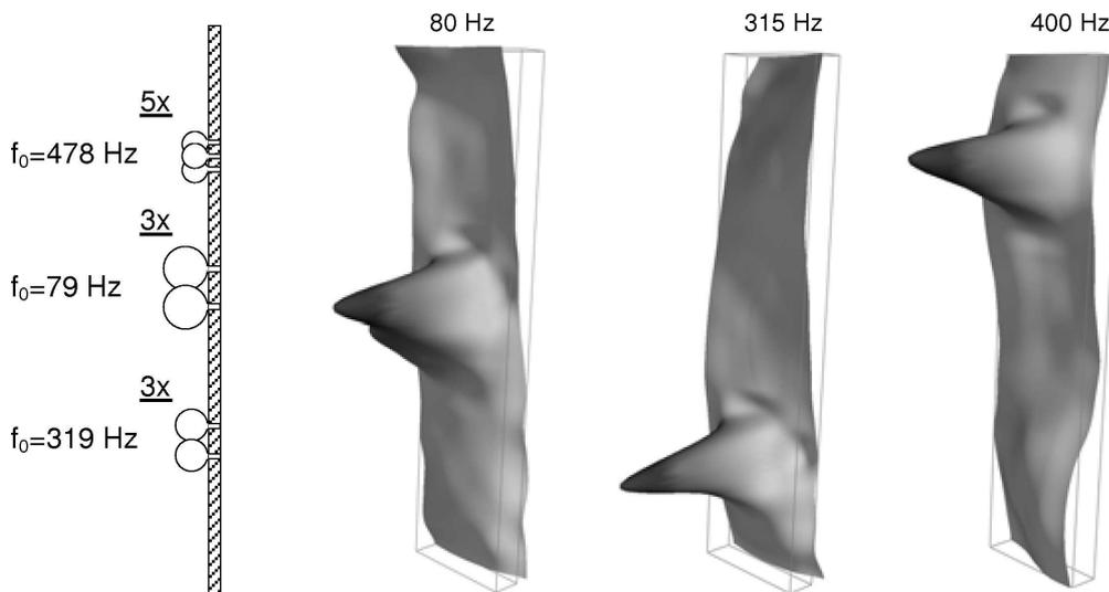
Fig. 4. Distribution of Helmholtz resonators in a simple suspended hard plate and graphic presentation of energy absorption by the separately groups of the resonators.
