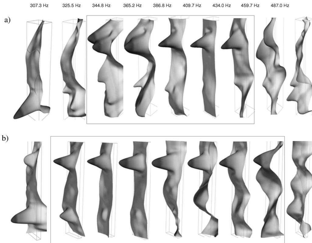
Fig. 5. The comparison of noise absorptions for the resonators ( $f_0 = 409$  Hz) in 1/12 octave band filters: a) filled with air, b) filled with rock wool ( $28 \text{ kg/m}^3$ ).
