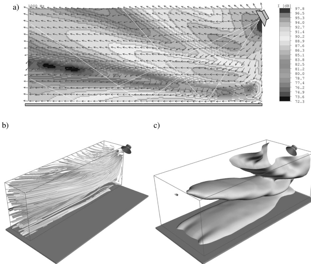
Fig. 6. Sound intensity wave reflected from a hard floor for, frequency  $f = 1000$  Hz: acoustic source – pink noise, loudspeaker oblige  $60^\circ$ , isosurface 88.5 dB.
