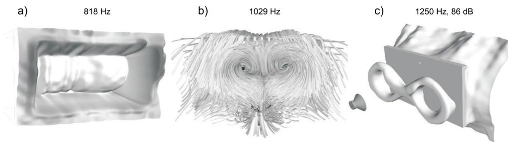
Fig. 2. The normal intensity component as a shape of wave (a) in a rear side of plate together with intensity streamlines (b) and intensity isosurface (c) for some selected frequencies.
