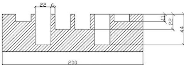
Fig. 1. Cross section of the test sample element. All dimensions given in mm.
