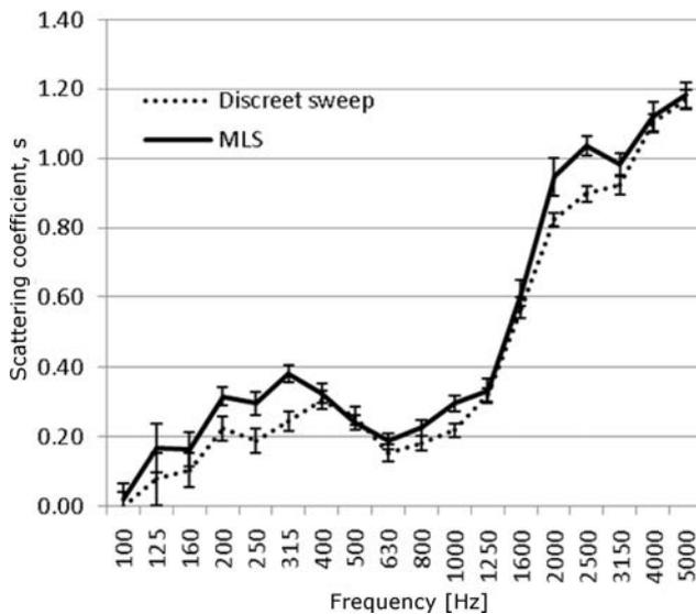
Fig. 7. Sound scattering coefficient from the measurement with a MLS signal (average value) and from discrete measurement using a sine sweep signal.
