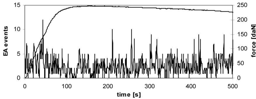
Fig. 4. Correlations between AE behaviour and the course of force during the PL effect in a tensile test of PA2 alloy predeformed by  $n = 6$  passes of the ARB method.
