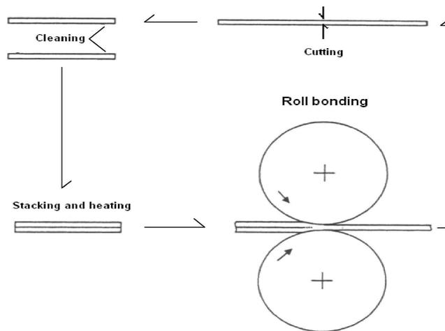
Fig. 1. Scheme of the accumulative rolling ARB.
