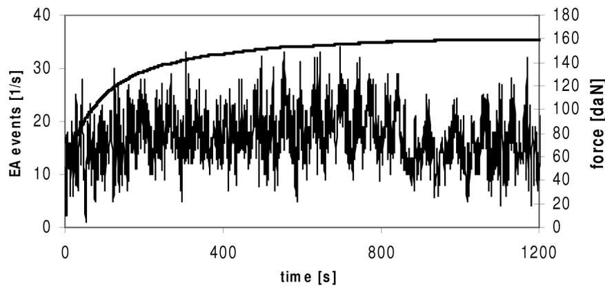
Fig. 2. Correlations between the AE behaviour and the course of force during the PL effect in a tensile test of PA2 alloy before the application of ARB operation.
