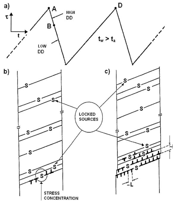
Fig. 6. Simple DD model of the PL effect [11]: a) jump-like drop of force, b) localization and nucleation of a slip band and c) propagation of a slip band.
