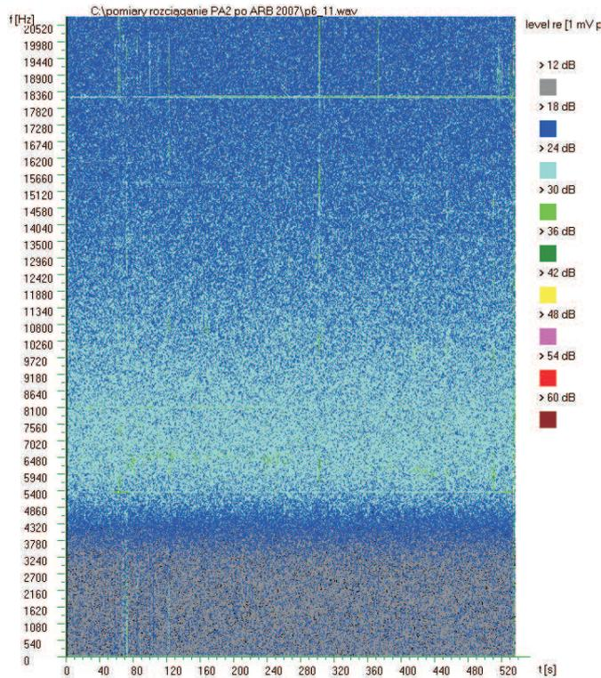
Fig. 5. Acoustic map of AE signals generated during tension of PA2 alloy after 6 repetitions of ARB operation.
