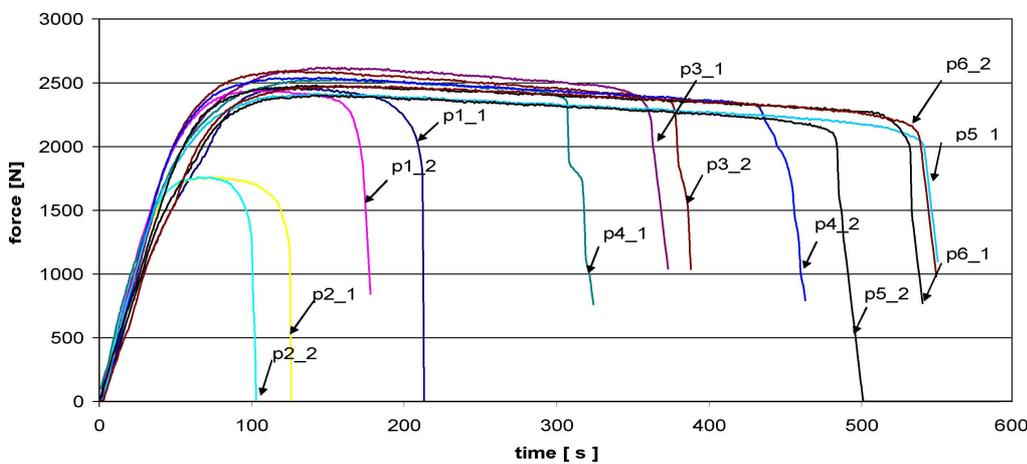
Fig. 3. Tensile curves in the force-time version for PA2 alloys obtained after  $n = 1$  to  $n = 6$  passes by means of the ARB method. There can be seen two series of curves illustrating good repeability of the measurements results.
