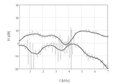
Fig. 10. Frequency response: fine line - FFT result, heavy line - averaged FFT result.
