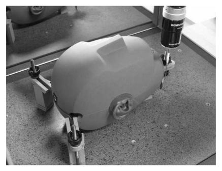
Fig. 3. Dummy head KU 100 in 3-D scanner holder.
