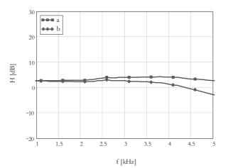
Fig. 6. Comparison of model responses for response pick up points located inside pinna (a) and outside pinna (b). Ipsilateral ear.
