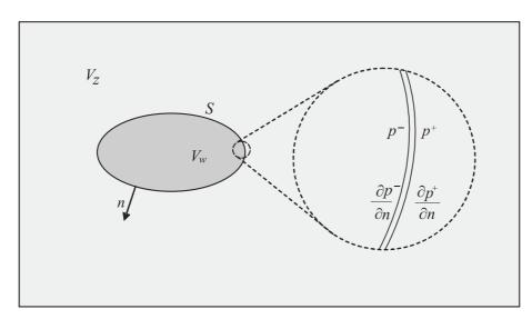
Fig. 9. Discontinuity of acoustic pressure and acoustic pressure derivative [16].
