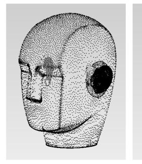
Fig. 4. Cloud of points – result of object measurement by means of 3-D scanner.
