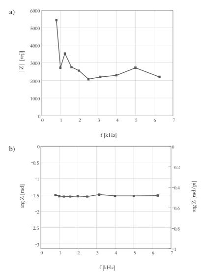
Fig. 8. Acoustic impedance of KU 100 a) modulus b) phase.
