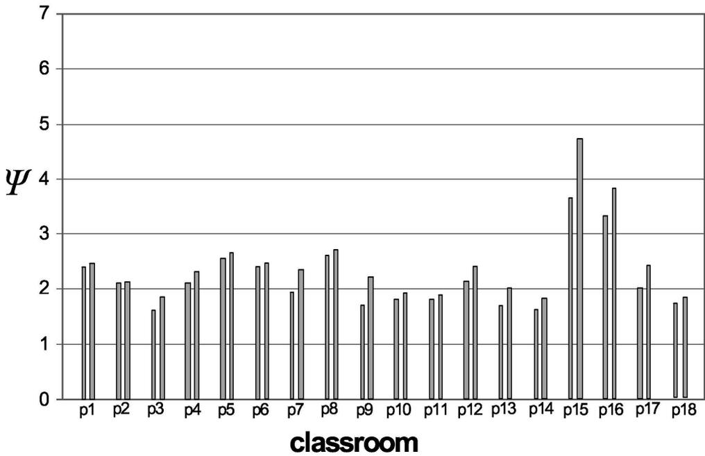
Fig. 2. Statistical fluctuation in frequency spacing for two frequency ranges: for the twenty-five lowest eigenmodes and up to the Schroeder frequency (parameter  $A$ ).
