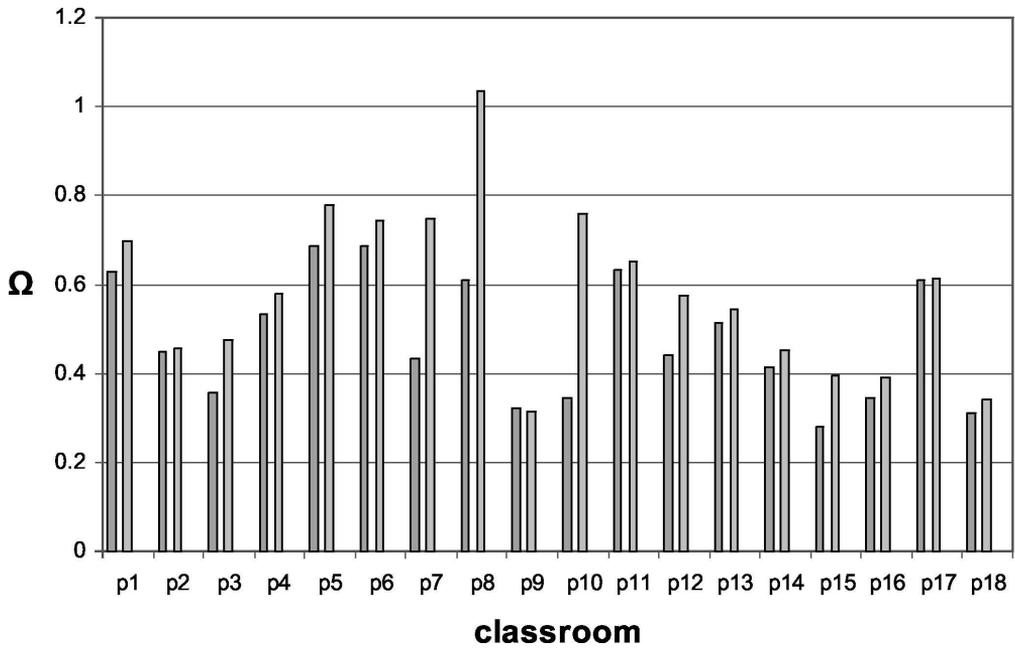
Fig. 4. Calculated values of  $\Omega$  for the 25 lowest eigenmodes and for frequencies up to the Schroeder frequency (parameter  $B$ ).
