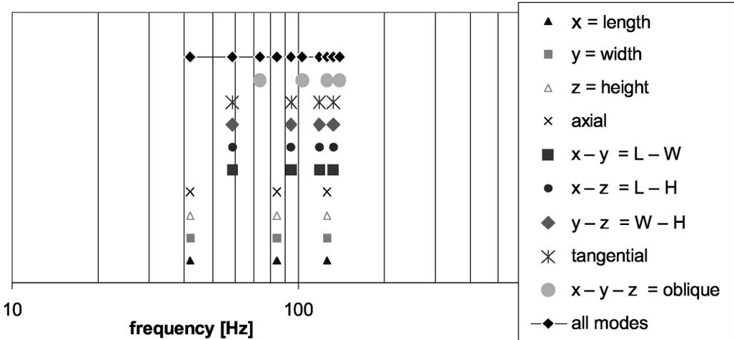
Fig. 3. Frequency spacing in a cubic enclosure (p15).
