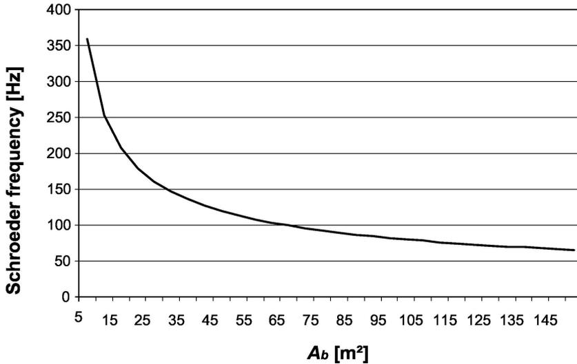
Fig. 1. Schroeder frequency [Hz] versus acoustic absorption [m<sup>2</sup>].
