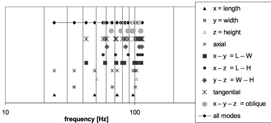
Fig. 5. Frequency spacing in room (p3).
