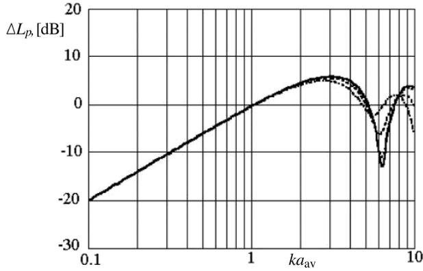
Fig. 3. Diffractive correction as the function of normalized wave parameter  $ka_{av}$  for loudspeaker placed in the center of rectangular baffles with  $B = 1$  (square, continuous line),  $B = 1.2$  (dotted line),  $B = 1.5$  (dashed line) and  $B = 2$  (dashed-dotted line).
