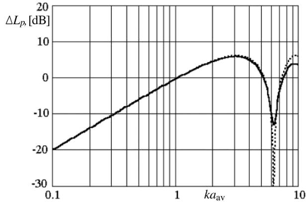
Fig. 2. Diffractive correction of the loudspeaker in the square baffle as the function of the normalized parameter  $ka_{av}$ . For comparison the correction of loudspeaker in the center of circular baffle of radius  $a$  ( $a_{av} = a$ ) is presented (dotted line).
