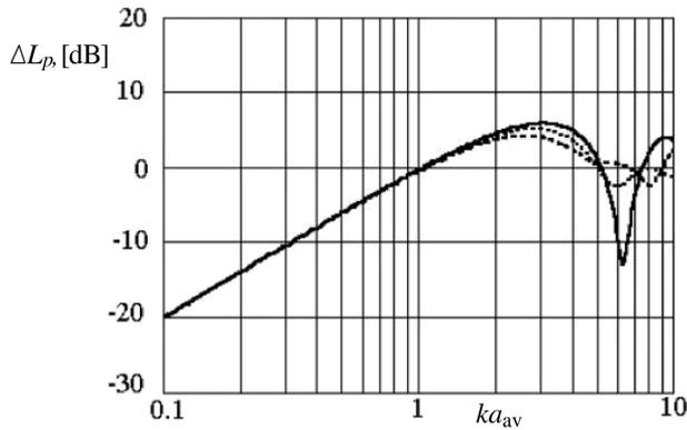
Fig. 4. The diffractive corrections for loudspeakers placed eccentrically in the rectangular baffles:  $B = 1.2, \xi_0 = 0.3, \eta_0 = 0.2$  (dotted line),  $B = 2, \xi_0 = 0.5, \eta_0 = 0.3$  (dashed line). For comparison – the correction of loudspeaker in the the square baffle (continuous line).
