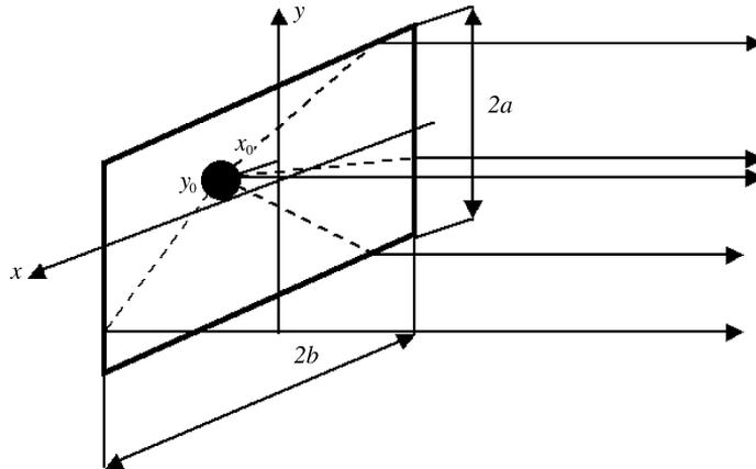
Fig. 1. The sketch for calculation of diffraction correction of loudspeaker in finite rectangular baffle.
