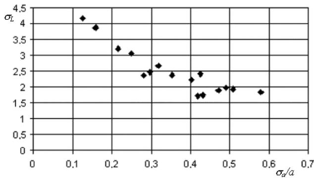
Fig. 5. Dependence between the standard deviation of the diffractive correction in the range  $1 < ka_{av} < 10$  and normalized standard deviation of the diffractive path around the baffle.
