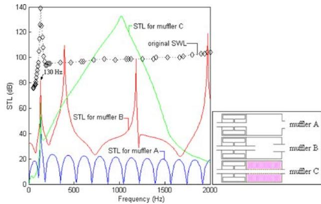
Fig. 7. Comparison of the original  $SWL$  (hybridized with a pure tone – 130 Hz) with respect to the  $STL$  at various mufflers [muffler A; a one-chamber  $HR$  element and a one-chamber simple expansion element; muffler B; a one-chamber  $HR$  element and a one-chamber tube-extended element; muffler C; a one-chamber  $HR$  element and a one-chamber dissipative element].
