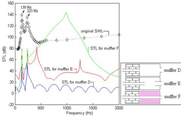
Fig. 8. Comparison of the original *SWL* (hybridized with two pure tone – 130 Hz and 235 Hz) with respect to the *STL* at various mufflers [muffler D; a two-chamber *HR* element and a one-chamber simple expansion element; muffler E; a two-chamber *HR* element and a one-chamber tube-extended element; muffler F; a two-chamber *HR* element and a one-chamber dissipative element].
