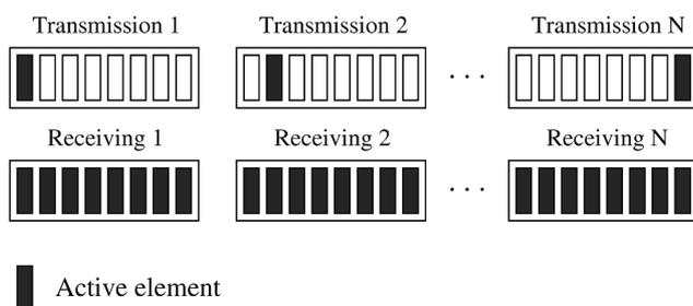
Fig. 1. Principle of the STA imaging method.
