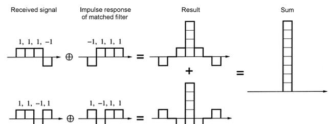
Fig. 2. Principle of side-lobes cancellation using a pair of Golay complementary sequences of the 4 bit length, where  $\oplus$  denotes correlation.
