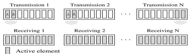
Fig. 5. Principle of the STA imaging method using mutually orthogonal Golay sequences for  $M = 2$ .
