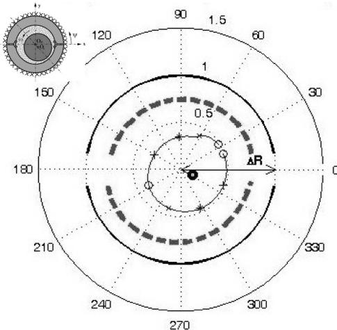
Fig. 7. Bush deformation (broken line) and journal trajectory (after exceeding the stability limit – continuous line – whipping of lubricating liquid –  $N = 6350$  rpm) for rigid external bush fixing.
