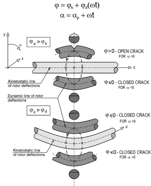
Fig. 3. The effect of kinetostatic rotor deflections on crack “breathing” process [1].
