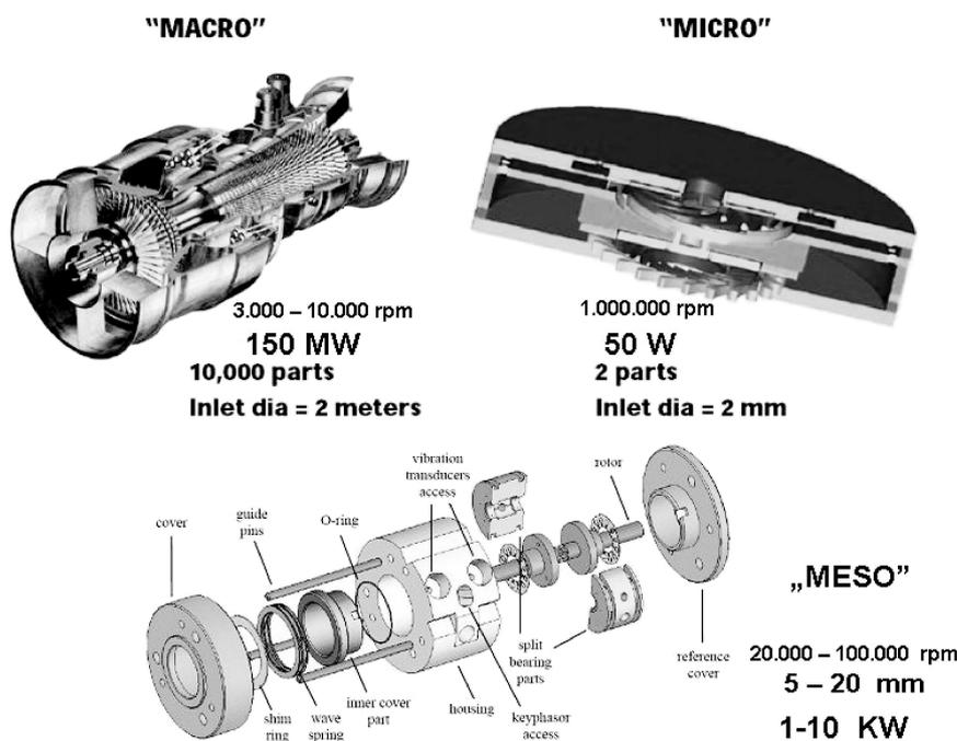
Fig. 1. Tendencies in development of turbines from MACRO through MESO to MICRO scale [2, 3].
