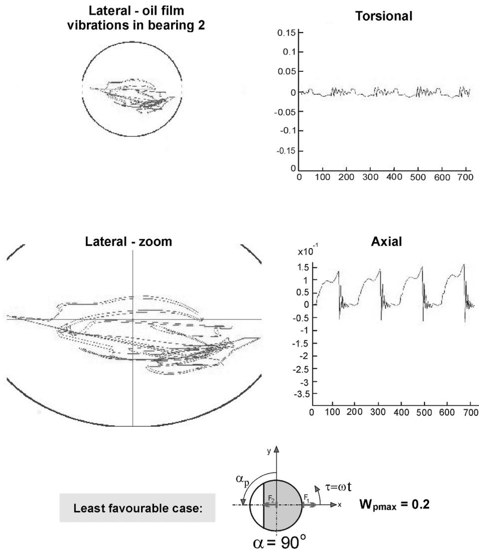
Fig. 11. Coupled vibration forms caused by the crack in resonance range  $N = 2600$  rpm (stable range of system operation). Circumferential crack position  $\alpha_p = 90$  – Fig. 5.
