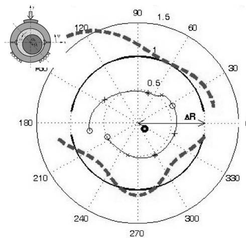
Fig. 8. Bush deformation (broken line) and journal trajectory (after exceeding the stability limit – continuous line – whipping of lubricating liquid –  $N = 6350$  rpm) for partial bush fixing with preliminary clamp.
