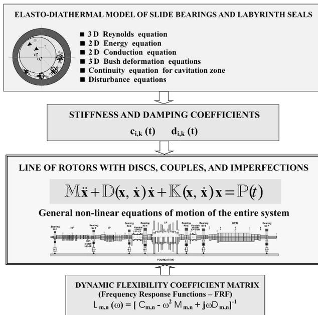
Fig. 4. Time-dependent slide bearing stiffness and damping coefficients, and the supporting structure dynamic flexibility matrices as the elements coupling together the main subsystems of the rotating machine, thus providing opportunities for solving mutually coupled ordinary and partial non-linear differential equations [1].
