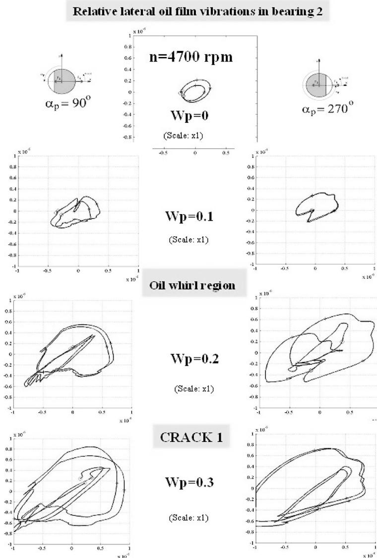
Fig. 13. The effect of rotor shaft crack propagation on the shape of lubricating liquid whirls, for two circumferential crack positions (after exceeding the stability limit  $N = 4700$  rpm).
