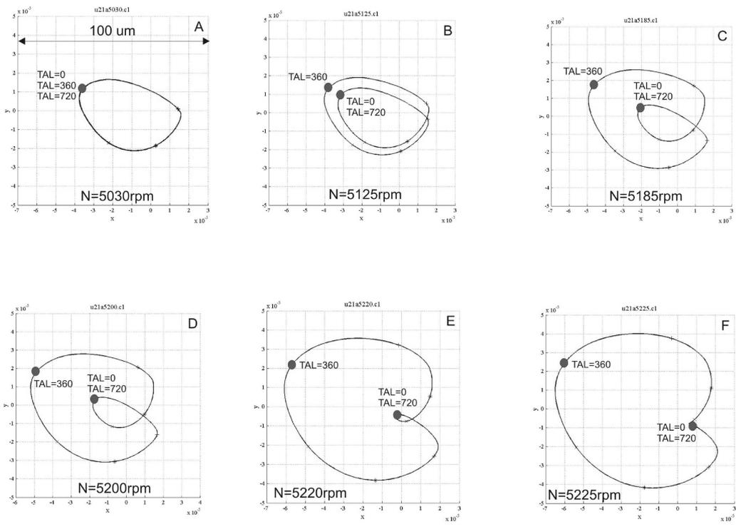
Fig. 10. Development of whirls in lubricating liquid after exceeding stability limit for partial fixing.
