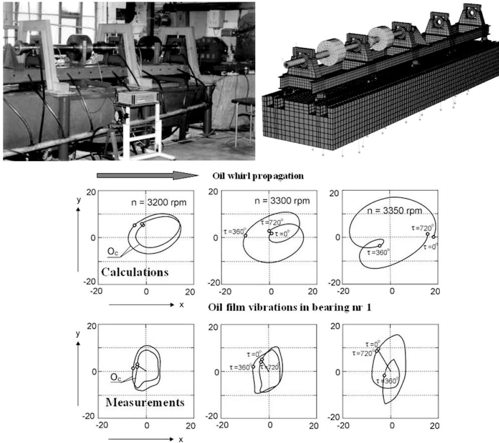
Fig. 6. Sample case of experimental verification of the computer system MESWIR on the research rig (photo taken in the IF-FM PAN vibrodiagnostic laboratory). Case of development of hydrodynamic instability (whirls).
