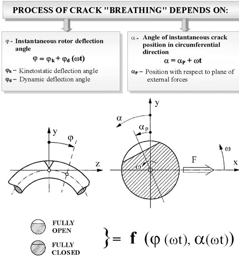
Fig. 2. The adopted concept of rotor shaft crack “breathing” process depending on instantaneous dynamic and kinetostatic positions [1].
