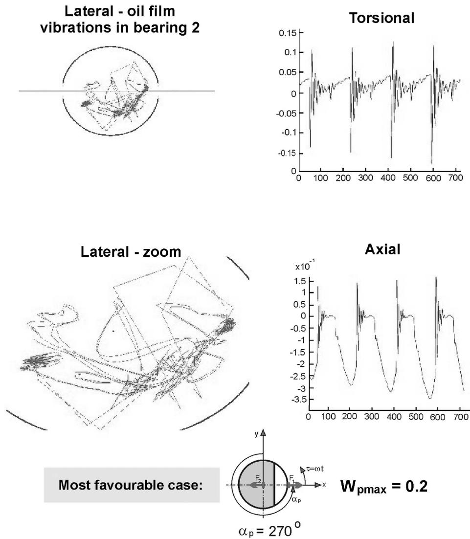
Fig. 12. Coupled vibration forms caused by the crack in resonance range  $N = 2600$  rpm (stable range of system operation). Circumferential crack position  $\alpha_p = 270$  – Fig. 5.
