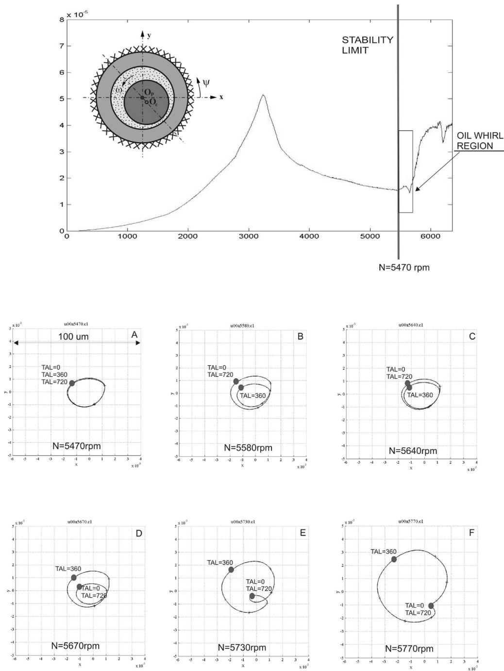
Fig. 9. Development of whirls in lubricating liquid after exceeding stability limit for rigid bush fixing.
