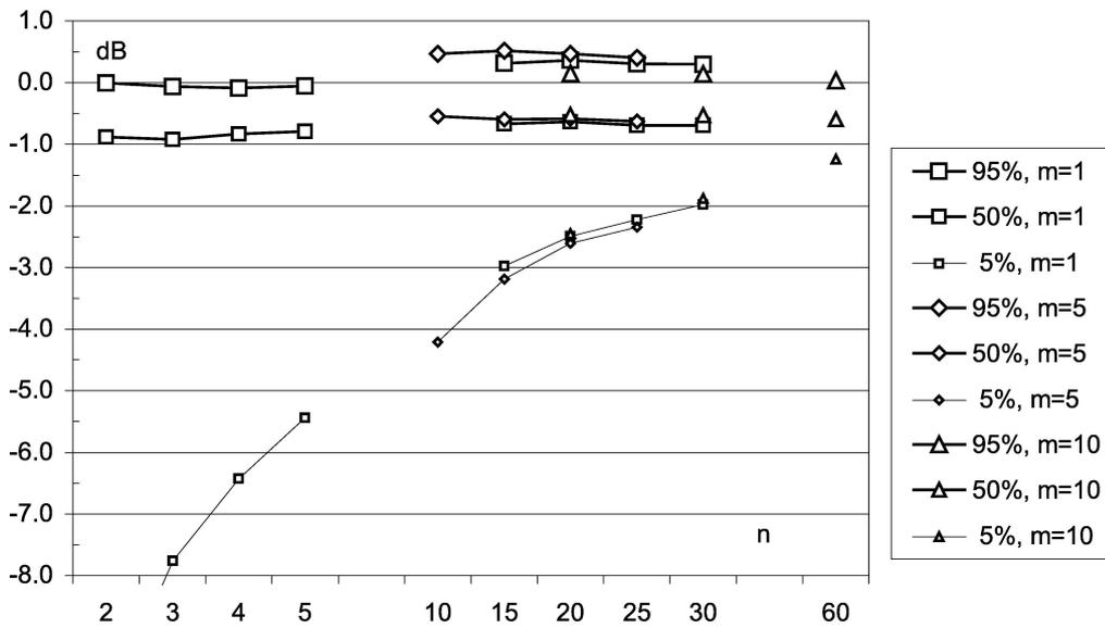
Fig. 1. Quantiles of  $\Delta L$  distribution, averaged values for 8 microphones.
