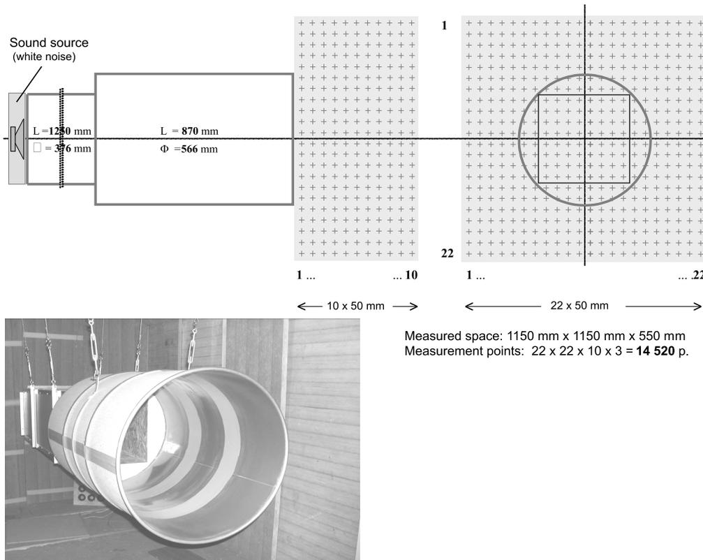
Fig. 1. The experimental facility sketch for study of outlet sound intensity distributions.
