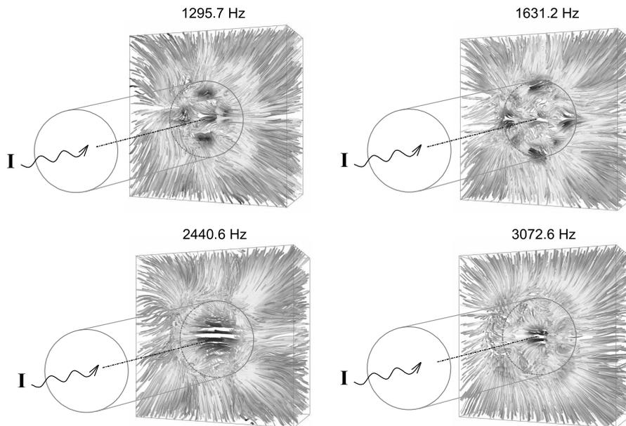
Fig. 3. Examples of intensity streamlines in the outlet region for some selected frequencies (shown from the rear side of measured space).
