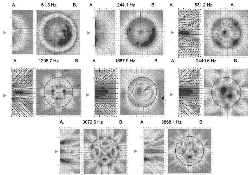
Fig. 2. Distribution of sound intensity field in the plane of symmetry axis of cylinder (A) and in the plane close to the outlet of cylinder (B).
