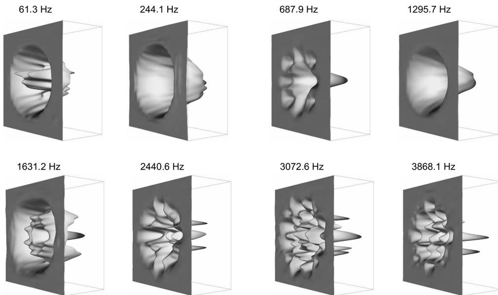
Fig. 5. Examples of the normal sound intensity component (as a shape of flow wave) in the measured plane close to end of cylindrical pipe.
