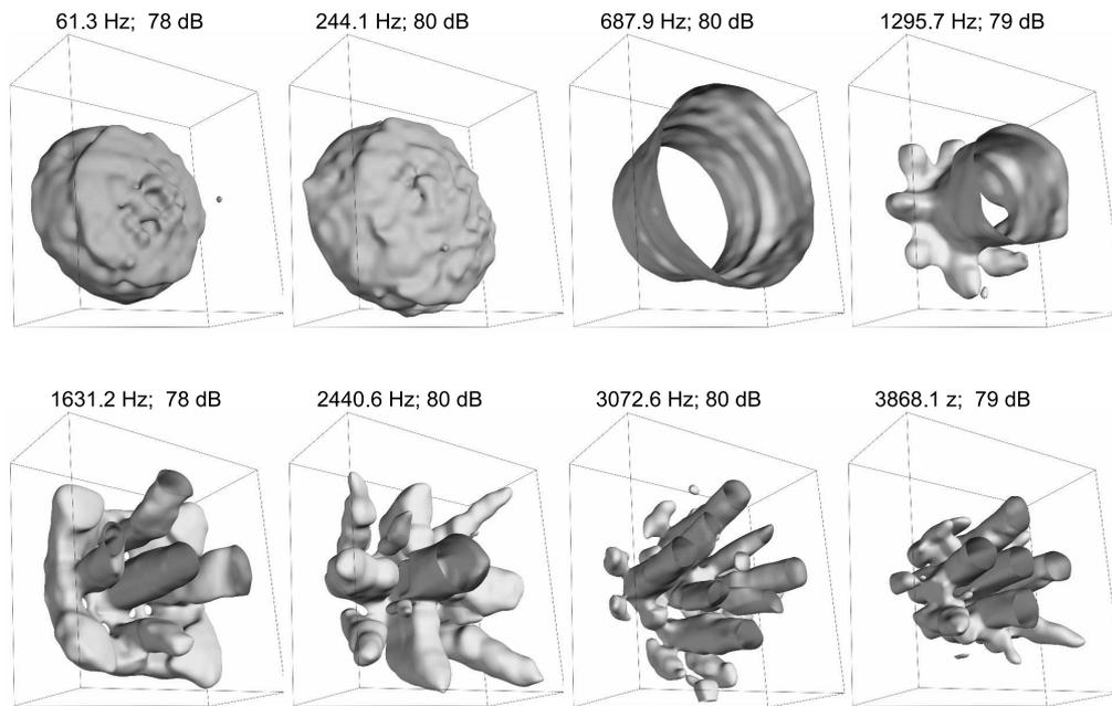
Fig. 4. Examples of intensity isosurface in the outlet region of cylindrical pipe for selected frequencies and levels of sound intensity.
