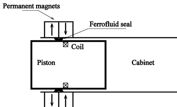
Fig. 1. Loudspeaker principle.
