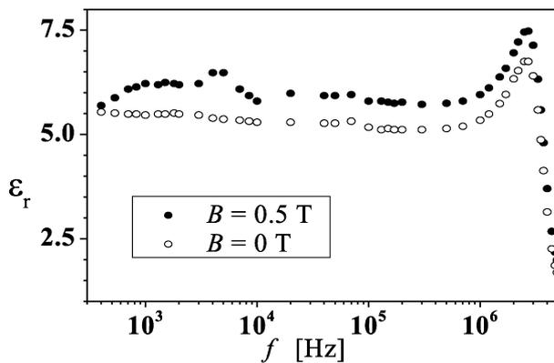
Fig. 1. Dispersion of dielectric permittivity of the PDMS ferrogel. The axis of the sample parallel to  $B$ .
