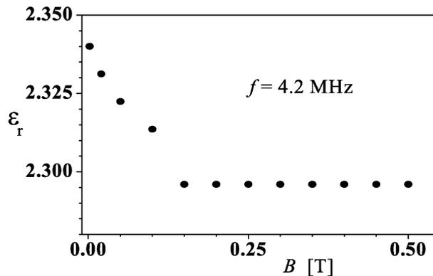
Fig. 2. Dielectric permittivity vs. magnetic induction  $B$ . The axis of the sample perpendicular to  $B$ .
