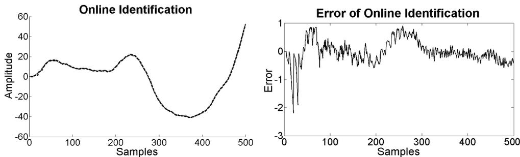
Fig. 3. Online identification process for 500 samples (sampling frequency: 25 kHz) ‘—’ output of real process, ‘- - -’ output of model.
