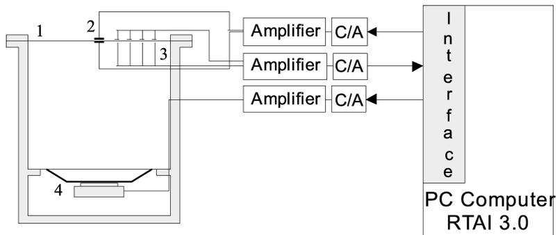
Fig. 1. Research position: 1 – circular plate, 2 – PZT elements, 3 – strain sensors, 4 – loudspeaker.
