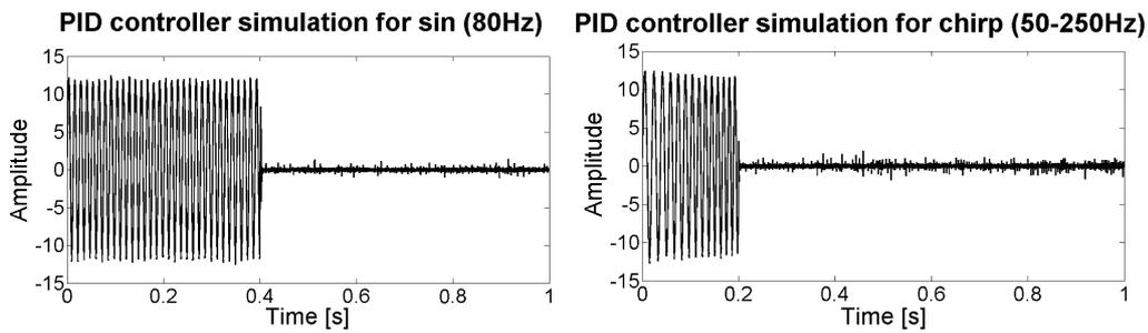
Fig. 4. Response of close-loop system with PID controller for *sin* and *chirp* signal (with noise).
