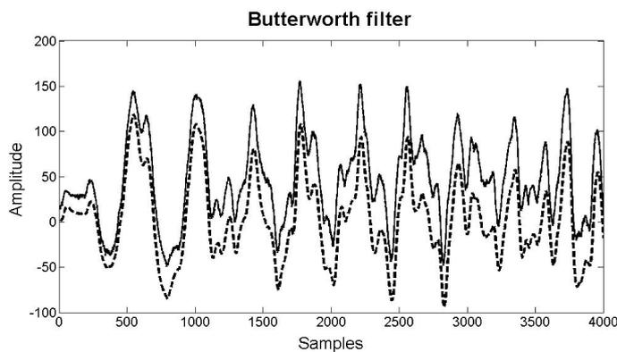
Fig. 2. Designed Butterworth filter filtering output data: ‘—’ real system output, ‘- - -’ filtered data.
