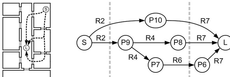
Fig. 5. Resulting transfer-path DAG (TP-DAG) for the sound source and listener in the example scene depicted in Fig. 3.
