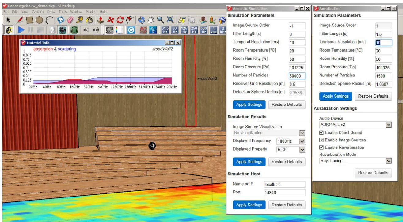
Fig. 8. Room acoustics simulation of a concert hall and calculation of room acoustical parameters using a plug-in for the CAD modeler SketchUp (PELZER *et al.*, 2014) that triggers the real-time room acoustics simulation framework RAVEN (SCHRÖDER *et al.*, 2010).
