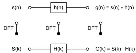
Fig. 2. Convolution of audio signals in time domain (top) or frequency domain (bottom).
