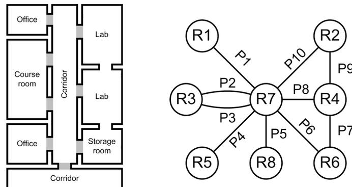
Fig. 4. The topological structure of the scene (acoustic volumes and their coupling through openings) in Fig. 3 described using an acoustic scene graph (ASG) (after WEFERS *et al.* (2009)).
