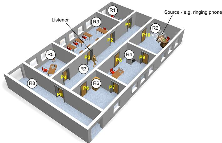
Fig. 3. An example scene with coupled rooms,  $R_1$ – $R_8$ , within an office building with coupling through portals  $P_1$ – $P_9$ , after WEFERS *et al.* (2009).
