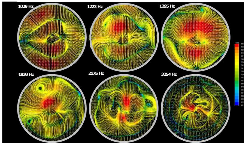
Fig. 4. The sound field in the cross section at 15 cm from the end of the waveguide – tumble motion as the effect of back-scattering reactions is shown.
