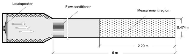
Fig. 1. Sound incident of circular cross section acoustic waveguide.
