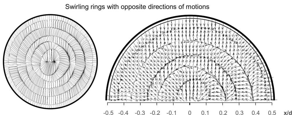
Fig. 3. Annula-helical coherent structure flow in-duct for 2440.62 Hz.
