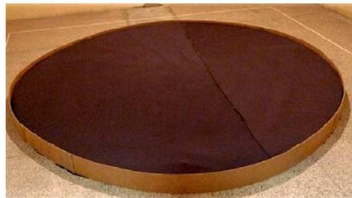
Fig. 2. The QRD covered with fabric used in the scattering coefficient measurement.
