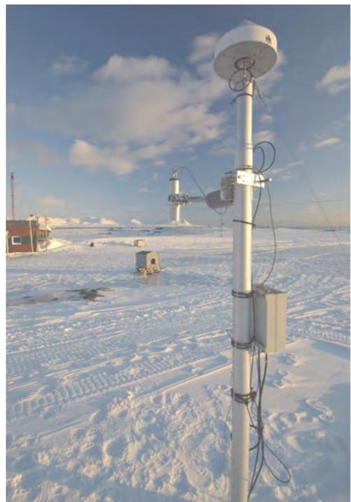
Fig. 11. Ultrasonic instrument measuring snow layer thickness mounted on a meteo mast during research on Spitsbergen.
