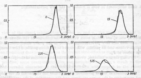
Fig. 3. The measured and calculated power spectra of the Doppler signal for flow with the Reynolds number Re = 1450. Thick line — measurements, thin line — calculations
