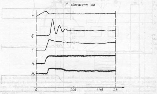
Fig. 9. Curves of changes in the pressure P and the air flow rates and sound levels:  $F_1$  — air flow rate at the inlet to the instrument,  $F_2$  — at the outlet,  $N_1$  — the mouthpiece vibration amplitude,  $N_2$  — sound amplitude at the outlet from the instrument
