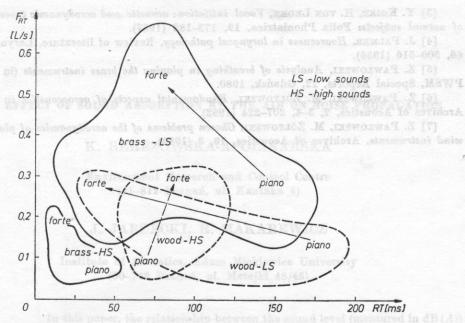
Fig. 12. Variability ranges of the air flow rates and rise times for the two groups of instruments
