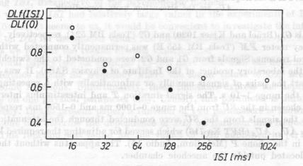
Fig. 2. The ratio DLf(ISI)/DLf(0) as a function of the interstimulus interval  $ISI. \circ$  and  $\bullet$  are for the signal durations T=32 ms and T=64 ms, respectively
