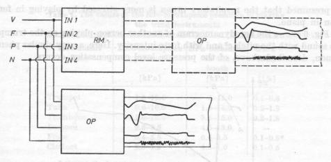
Fig. 4. A schematic diagram of the system for the recording of the measured quantities from the examinations. V — the volume, F — the flow, P — the pressure in the oral cavity, N — the sound intensity level, RM — the magnetic recorder, OP — the loop oscillograph, — variant I, — — — variant II
