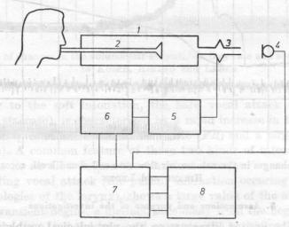
Fig. 4. A schematic diagram of the measurement system: 1. instrument encasing, 2. instrument, 3. pneumotachometer, 4. microphone, 5. flow signal amplifier, 6. electronic spirometer, 7. magnetic recorder, 8. multi-channel recorder
