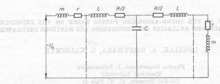
Fig. 1. An equivalent electric system of the two-sided perforated sound-absorbing panel
