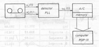
Fig. 2. A schematic diagram of the measurement system for the calculation of a listogram of the instantaneous frequencies of a Doppler signal
