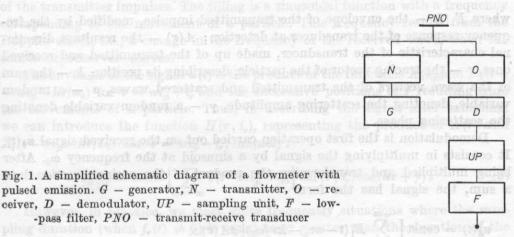
Fig. 1. A simplified schematic diagram of a flowmeter with pulsed emission. G – generator, N – transmitter, O – receiver, D - demodulator, UP - sampling unit, F - low--pass filter, PNO - transmit-receive transducer
