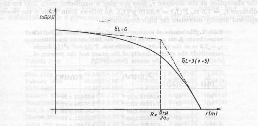
Fig. 2. Sound level drop  $\delta L$  for a double distance for  $r \leqslant R$  and  $r \geqslant R$ , where R is the "critical distance" (formula (12))
