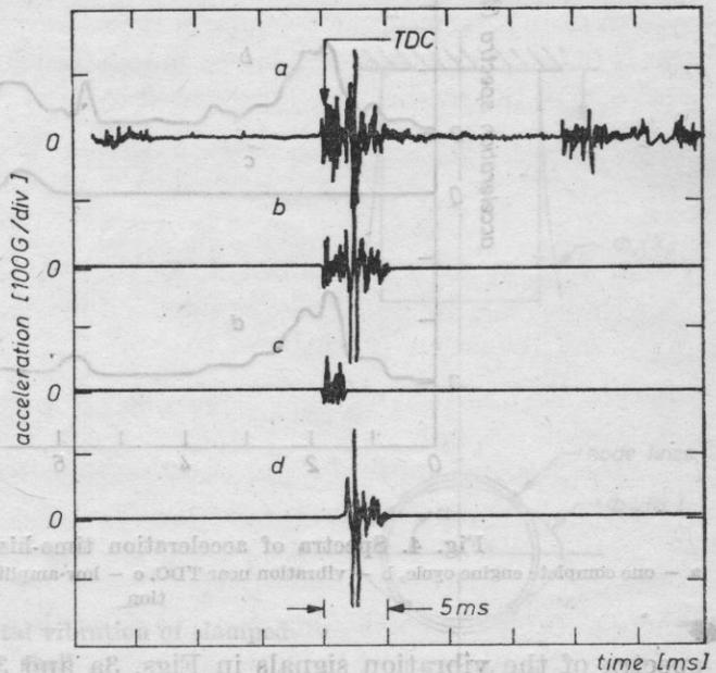
Fig. 3. Typical cylinder liner acceleration time-histories
