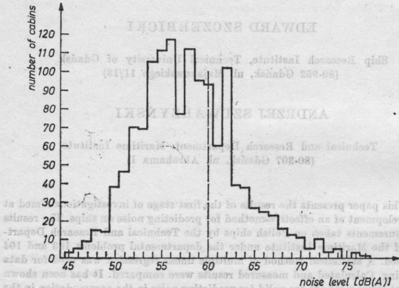
Fig. 1. The distribution of noise levels in accommodations in the ships of PLO and PŻM
