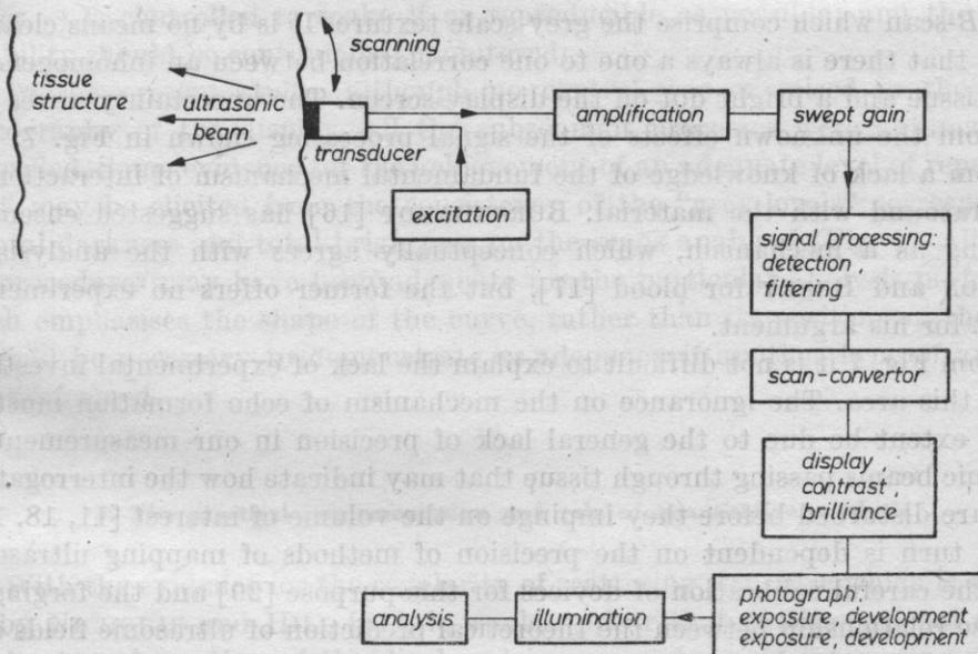
Fig. 7. Factors in ultrasonic imaging that may affect the results in the type of image analysis proposed
