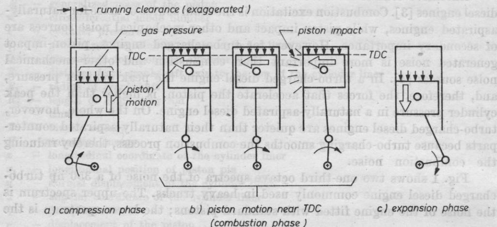
Fig. 2. Sequence of events showing piston-impact phenomenon
