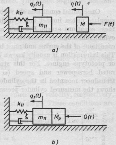
Fig. 6. Models for piston impact and cylinder liner vibration
