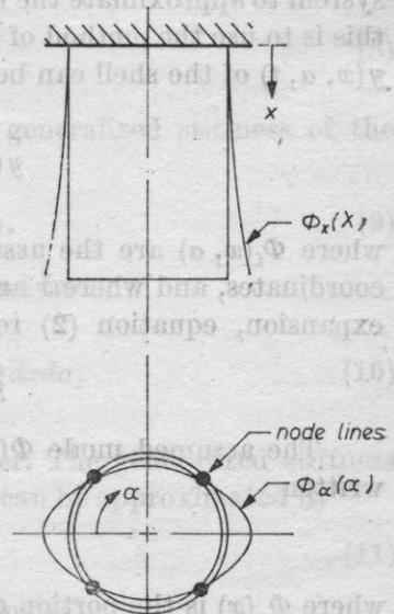
Fig. 5. Mode shape for fundamental vibration of clamped-free cylindrical shell
