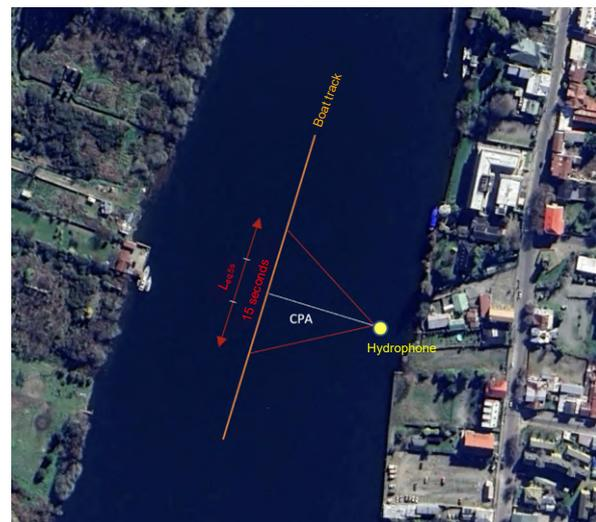
Fig. 5. The orange line shows the boat track in front of the hydrophone and the yellow circle indicates the hydrophone position.
