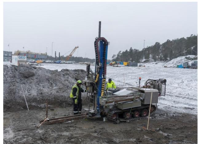
Fig. 1. Process of CPT sounding in Norvik area.
