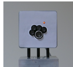
Fig. 11. Sonar module used in experiments.
