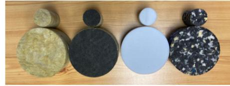
Fig. 1. Material specimens of mineral wool (MW151), mineral wool with glass fleece (MW100), melamine foam (ME), and rebonded polyurethane foam (PU).
