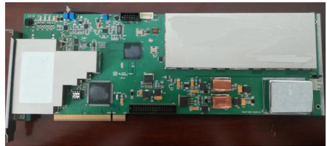
Fig. 2. Ultrasonic flaw detection card.
