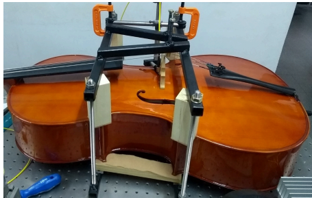
Fig. 2. Cello mounted on the measuring table by means of the clamping frame.
