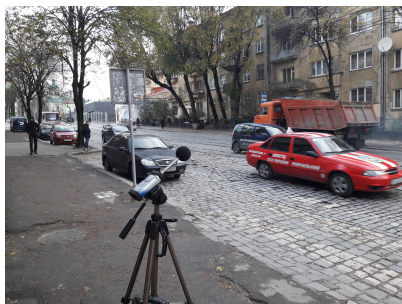
Fig. 2. Measurement of the equivalent noise level during the day on Taras Shevchenko Street.
