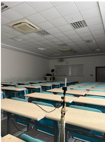
Fig. 8. Experimental study conducted in classroom A203, microphone position: R3, temperature: 26.5 °C.
