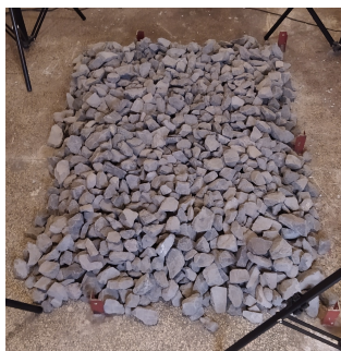
Fig. 5. Ballast layer (stone aggregate, grain size 31.5/50 mm).
