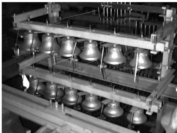
Fig. 3. The twelve, new installed carillon bells (control levers of mechanical action are visible).
