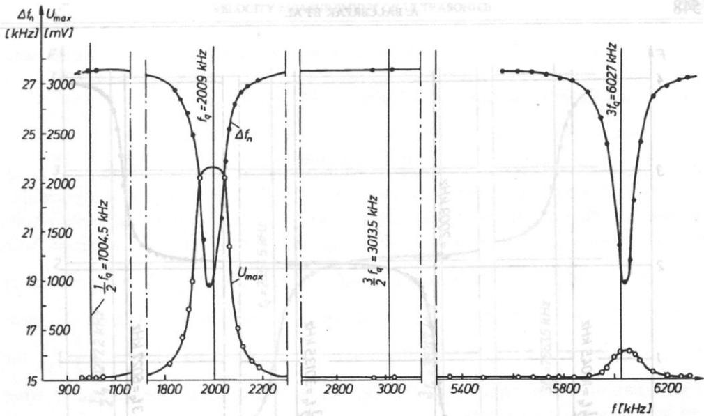
Fig. 6. The frequency intervals  $\Delta f_n$  and maximum amplitude of the output signal at resonances  $U_{max}$  as a function of the frequency  $f$  for the cell No. 2. The 20 mm distance ring. Methanol.  $f_q = 2009$  kHz,  $l = 20.06$  mm,  $f_1 = 27.571$  kHz,  $U_{input} = 5.8$  V.
