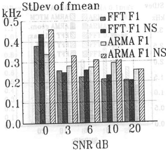
Fig. 8. Bias and standard deviation of  $f_{mean}$  for wide-band signal with Gaussian envelope spectrum computed using first moment F1 with and without noise suppression NS, SNR changes from 0 to 20 dB.
