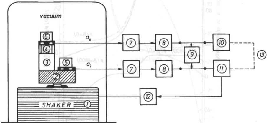
Fig. 6. Measuring arrangement 1. shaker; 2. table; 3. specimen; 4. loading mass; 5. control accelerometer; 6. pickup accelerometer; 7. amplifier; 8. filter; 9. phase meter; 10. level recorder; 11. sinusoidal generator; 12. power amplifier; 13. mechanical linkage.
