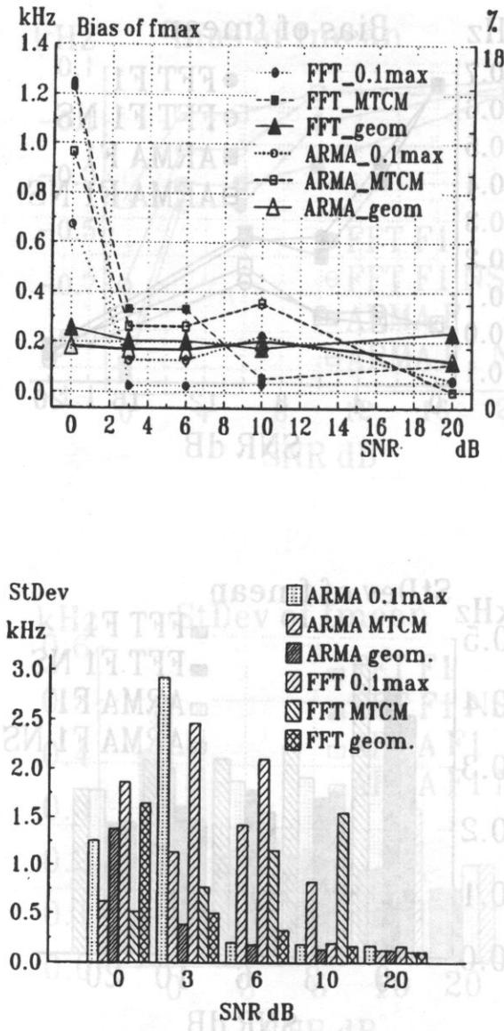
Fig. 9. Bias and standard deviation of  $f_{max}$  for narrow band signal with Gaussian envelope spectrum computed using 0.1max, MTCM and geometrical methods, SNR changes from 0 to 20 dB.
