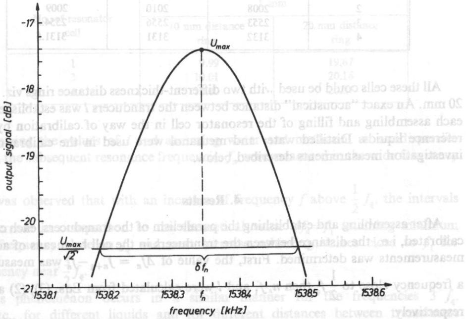
Fig. 3. The resonance curve for the frequency  $f_n = 1538,342$  kHz.
