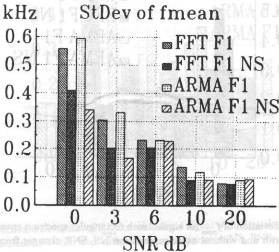
Fig. 6. Bias and standard deviation of  $f_{mean}$  for narrow band signal with Gaussian spectrum envelope computed using first moment F1 with and without noise suppression NS, SNR changes from 0 to 20 dB.
