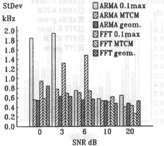
Fig. 11. Bias and standard deviation of  $f_{max}$  for the signals with wide-band Gaussian spectrum envelope computed using 0.1max, MTCM and geometrical methods, SNR changes from 0 to 20 dB.
