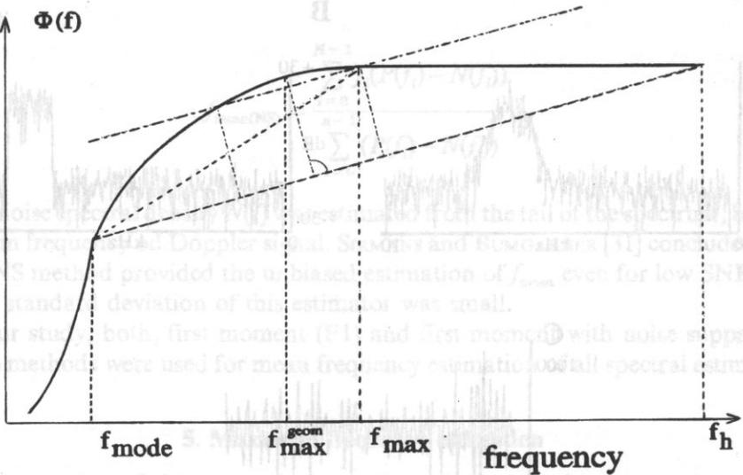
Fig. 3. Principle of the geometrical method used for calculation of  $f_{max}$
